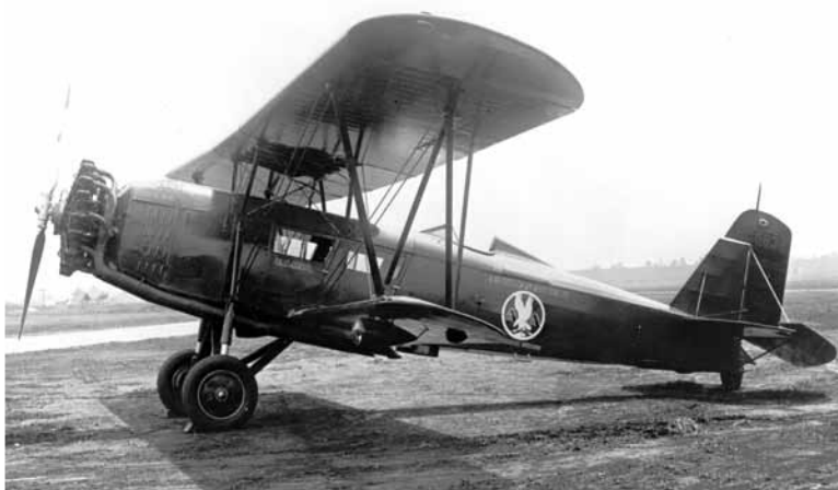
Stearman LT-1, NC8832, in service with the Universal Division of American Airways. Big, four-passenger ship with 525-hp P&W Hornet was originally built for Interstate Airlines; used for combined mail and passenger operations. (Photo courtesy American Airlines)
