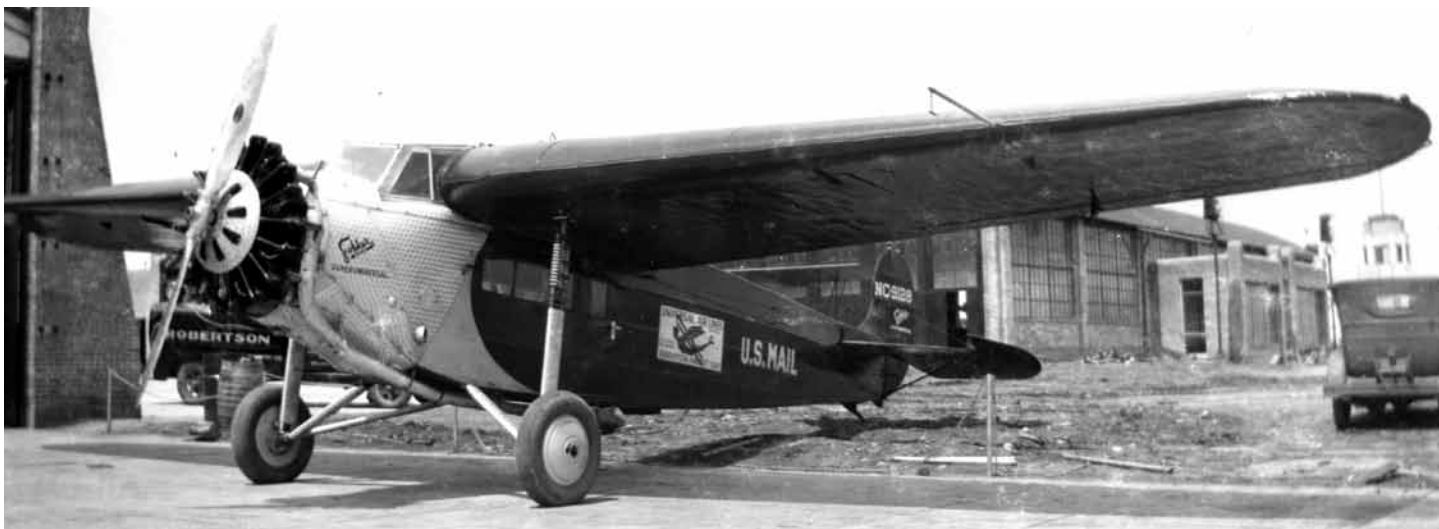
Fokker Super Universal NC9128 on the Universal ramp at Lambert Field. This six-passenger Wasp-powered transport had the reputation of being very stable and a fine instrument ship. Unfortunately, the casein-glued plywood wings did not weather well, so the aircraft were retired after a relatively short service life. (Photo by Vic Stuhr)
