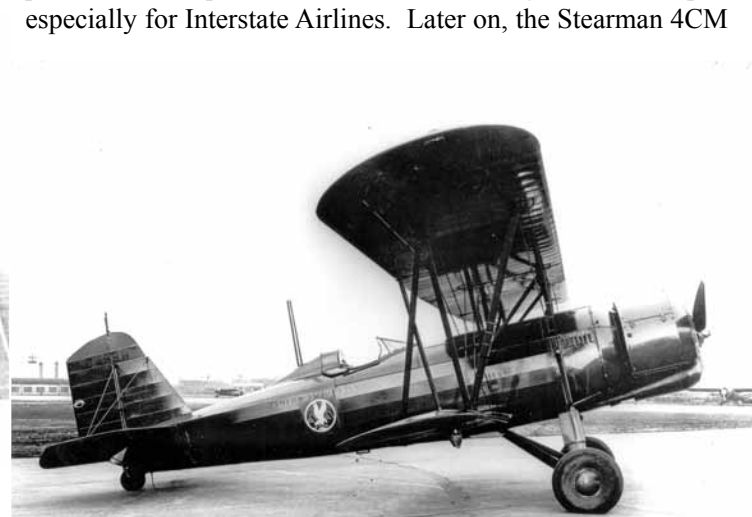
Stearman 4CM Junior Speedmail, NC469W, was powered by a 300-hp J6 Whirlwind. This ship was operated over the Interstate Division of American Airways during 1929-30, carrying mail only. (Photo courtesy American Airlines)
