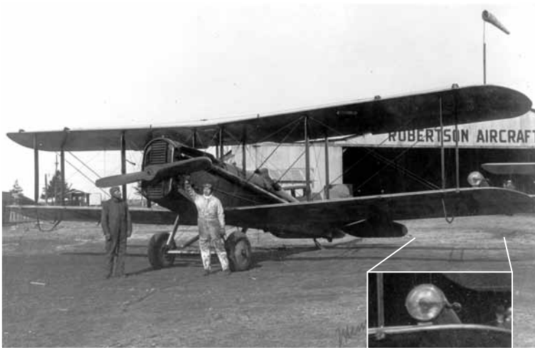
The workhorse of CAM-2 airmail service was the big DH-4, a WWI aircraft converted for airmail use. Inset: Note the landing lights on the upper side of the lower wing.
