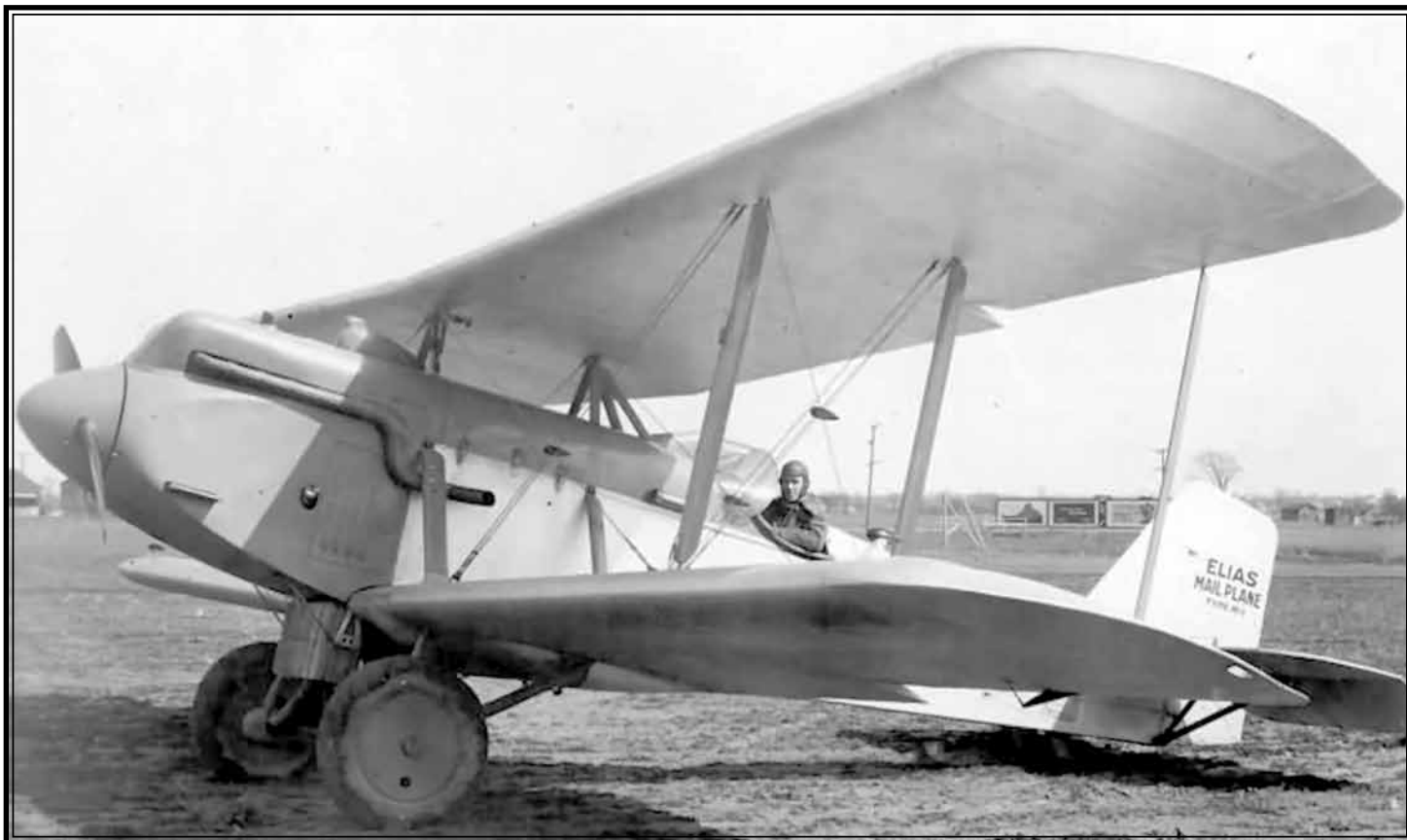
Quarter front view of the Elias M-1 showing the clean design and the accessible mail compartment and engine. (Substitute photo from the Jesse Davidson collection via Dan Shumaker and 1000AircraftPhotos.com)
