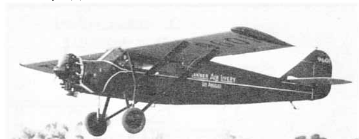
SM-1DA DETROITER (6PCLM, 220-hp Wright J5C). Same as SM-1 except for minor changes. 1928 production; 5 built under ATC 74: s/n 300, 302, 304 thru 306.
