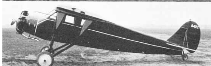
SM-2AA JUNIOR (4PCL, 175-hp Wright R540). 1929 production; 25 built under ATC 145: s/n range 1046 thru 1126.
