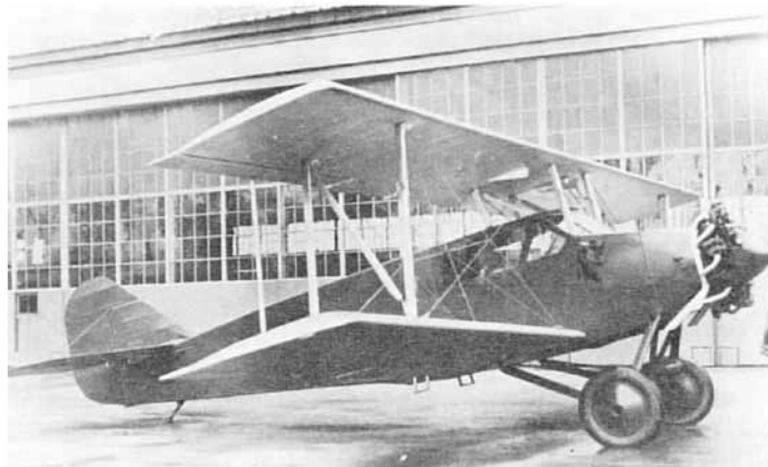
SB-1 DETROITER (5PCL/SB, 200-hp Wright J4B or 220-hp J5C). Developed from preceding aircraft; 1926-27 production 26 built: s/n 1 thru 5, 10, 30, 70, 80, 90, 102 thru 117 and 201-B. First production model by Stinson. Retroactive certification under ATC 24. Users: Northwest Airways (3), Wayco Air Service (3), Patrician Airways Ltd (3), Florida Airways (2).
