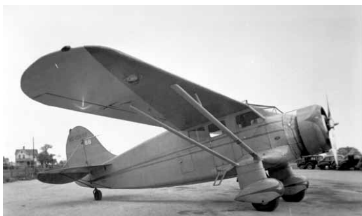
MODEL "R" (4PCLM, 215-hp R680). Extensive redesign of SM-8/Model S by C.R. Irvine and R.W. Ayer. 1932 production; 31 built under ATC 457: s/n 8500 thru 8533. R-2 (4PCLM, 240-hp R680-BA). 3 built under ATC 493: s/n 8500, 8512 and 8521.
