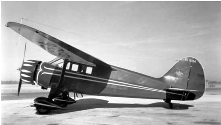
SR-8D RELIANT (5PCL/SM, 285-hp Wright R760E1). 11 built under ATC 609: s/n range 9727 thru 9795.
