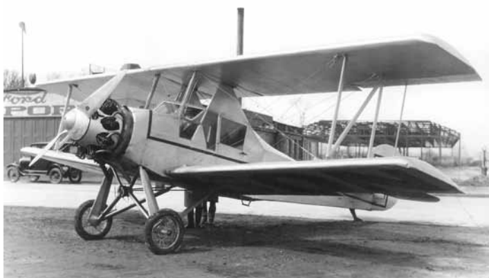
DETROITER (4/5PCLB, 200-hp Wright J4B). First Detroit-built Stinson; designed by E.A. Stinson with engineering by Prof. Peter Altman. Reputedly first cabin plane with brakes and starter. Initially tested January 1926.
