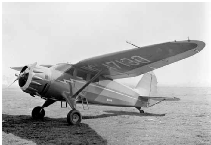
SR-9D RELIANT (5PCL/SM, 285-hp Wright R760E1). 22 built under ATC 625: s/n range 5217 thru 5223S, 5250 thru 5271, 5454, 5455. One USAAC impressment as UC-81G.
