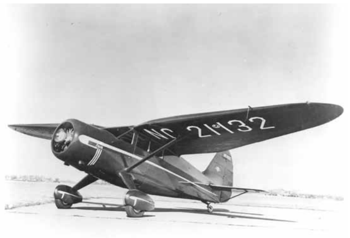
SR-10C RELIANT (5PCL/SM, 260-hp R680-D5). Final refinement of the civil Reliant series under project engineer Gordon Isreal. 1938 (Series 5800) and 1939-40 production (Series 5900). 46 built under ATC 678: s/n range 5803 and 5855, 5901 thru 5930. Five USAAC impressments as UC-81K, 1942.
