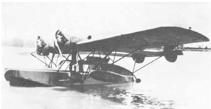
MODEL "A" (5PCAmM, 2 x 215-hp R680). 1931 experimental amphibian; NX11117, s/n M-7000. Project abandoned after unsatisfactory testing.
