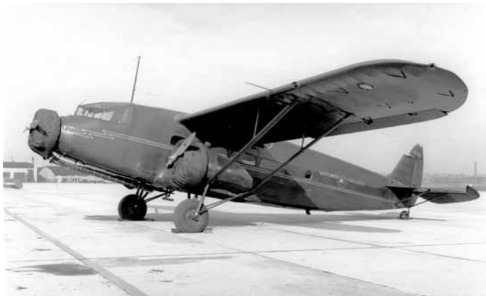
MODEL "U" (12PCLM, 3 x 240-hp R680-BA). Designed by Art Saxon as SM-6000B replacement. Prototype NC(X) 432M, s/n 9000, certificated under ATC 2-413; 1932-33 production, 20 built under ATC 484: 9001 thru 9012, 9015 thru 9023. Fleet users: AAL (16), Trans-American Airlines (1) and Iliolo-Negro Air Express (2). Experimental Model U, s/n 9013, with modified tail, destroyed in crash February 1933.
