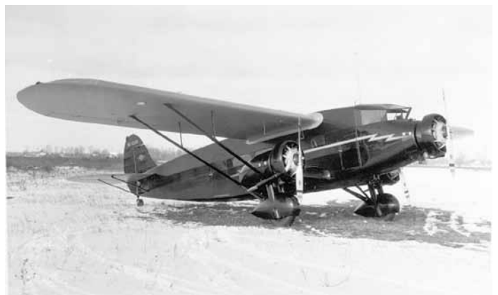
U-1 (11PCLM, 3 x 285 Wright R760E1). 1 built under ATC 2-437 for Eastern Air Transport: s/n 9014.
