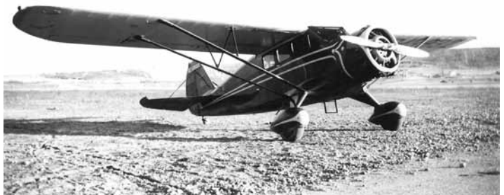
SR RELIANT (4PCL/SM, 215-hp R680). Redesign of Model R by C.R. Irvine. 1933 production; first of the Reliant series. 89 built under ATC 510: s/n 8700 thru 8788.
