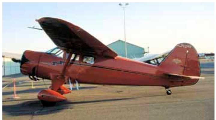
SR-9B RELIANT (5PCL/SM, 245-hp R680-D6). 1937 production; 35 built under ATC 621: s/n range 5100 thru 5123, 5151 thru 5173, 5300 thru 5325, 5353 thru 5365. One USAAC impressment as UC-81N, 1942.
