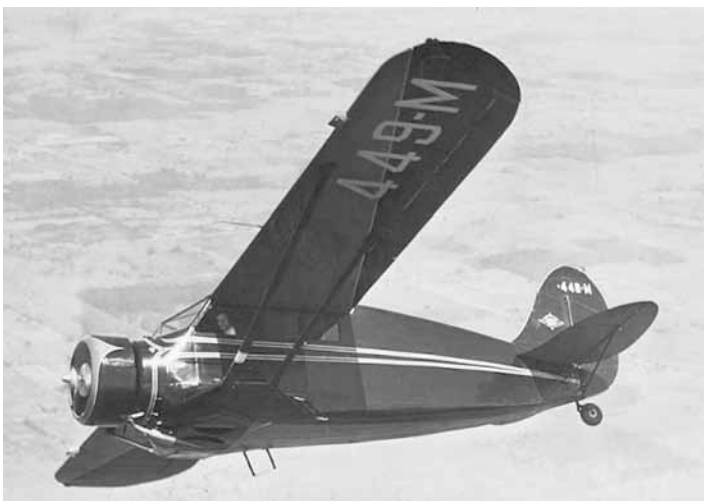
R-3 (4PCLM, 240-hp R680-BA). Same as R-2 except for retractable landing gear and minor changes.
