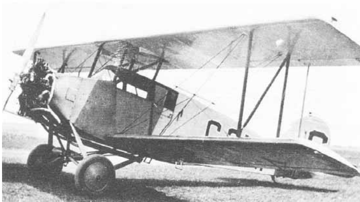
SM-1D-300 (6PCLM, 300-hp Wright R975A). No production; s/n 300 thru 307 eligible for factory conversion under TC 2-60.
