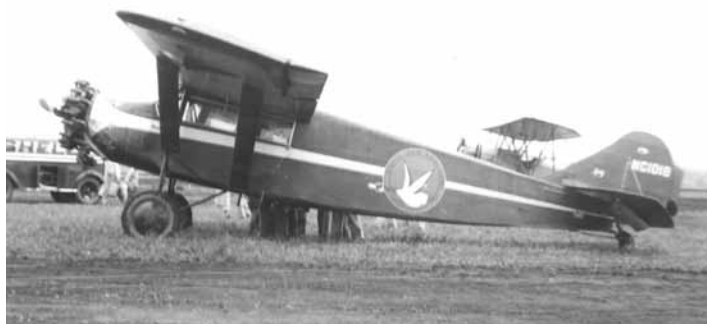
SM-1 DETROITER (6PCLM, 220-hp Wright J5C). Designed by W.C. Naylor to E.A. Stinson's requirements; prototype first flown April 1927. 1927-28 production under ATC 16. SM-1B Same as SM-1 except for minor changes, revised landing gear; 1928 production under ATC 2-24. Total 75 built; s/n 200 thru 205, 205A, 206 thru 273.
