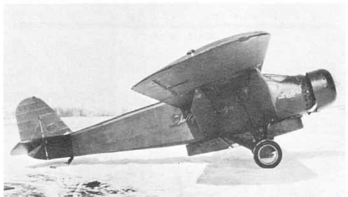
SM-4 (2PCLM, 300-hp Wright R975A). "Sally Sovereign," special endurance plane with retractable landing gear developed from SM-1. s/n X-10, X9696. Unsuccessful, revised as "K of New Haven," c. 1930.
