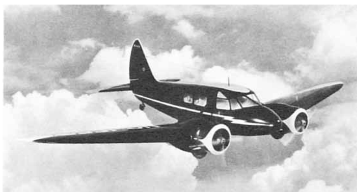
MODEL "B" (6PCLM, 2 x 245-hp R680-B6). Projected twin-engined executive aircraft based on Model A design. Mock-up only.
