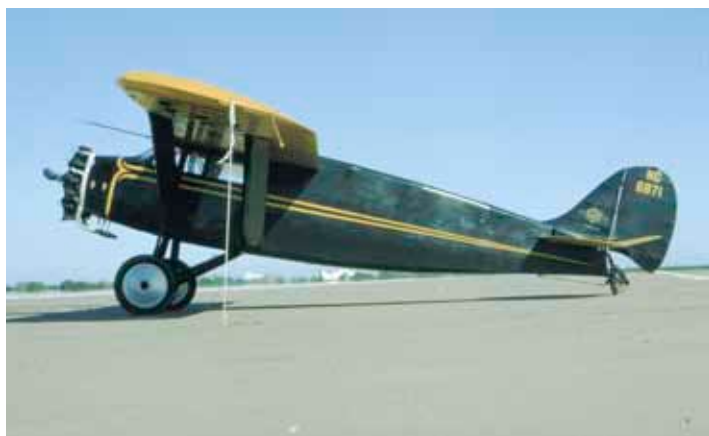
SM-2 JUNIOR (3/4PCLM, 110-hp Warner Scarab). Designed by W.C. Naylor for 1928 production. 42 built under ATC 48: s/n 1001 thru 1045.
