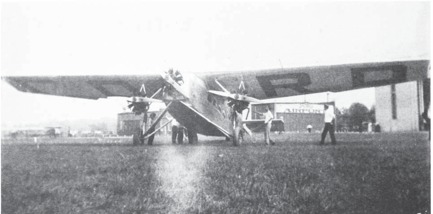
Above: The prototype 4-AT-1 with Wright J-4 engines of 200 hp and Curtiss-Reed propellers at Ford Airport, sometime between its original wing planform and the modification which moved the ailerons aft. Revision of landing gear to final configuration had not yet taken place.
