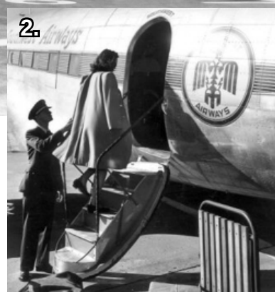
1. Southwest Airways DC-3, N63107, seen at Los Angeles (LAX) in 1952. Note the airstair door that this airline pioneered and that greatly assisted in reducing turnaround time at a station. This innovation would be widely adopted in various forms by other feeder lines. (From the Tim Williams collection) 2. Detail of airstair door. (From the Ed Coates collection via the author) 3. Southwest's "Family Plan" allowed family members to fly for half-fare. This promotion inspired cartoonist Wiley Smith to use this as a "foil" in this cartoon. (From the author's collection) 4. The Thunderbird logo for the airline incorporated into a baggage label. (From the author's collection)
