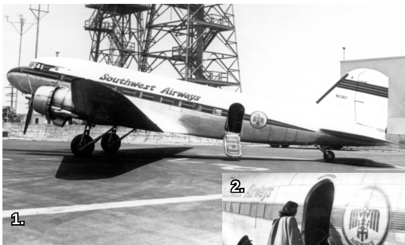
1. Southwest Airways DC-3, N63107, seen at Los Angeles (LAX) in 1952. Note the airstair door that this airline pioneered and that greatly assisted in reducing turnaround time at a station. This innovation would be widely adopted in various forms by other feeder lines. (From the Tim Williams collection) 2. Detail of airstair door. (From the Ed Coates collection via the author) 3. Southwest's "Family Plan" allowed family members to fly for half-fare. This promotion inspired cartoonist Wiley Smith to use this as a "foil" in this cartoon. (From the author's collection) 4. The Thunderbird logo for the airline incorporated into a baggage label. (From the author's collection)
