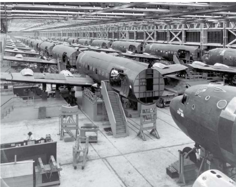
The assembly line in the Douglas Aircraft plant in Orchard Place on July 7, 1944, where wings are attached to the fuselage of big C-54 cargo planes. The plant was 15 percent ahead of schedule in June 1944. (Douglas Aircraft photo)
