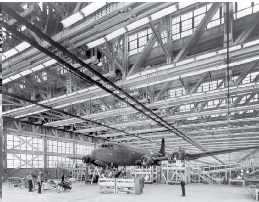
Douglas C-54 in final assembly at the Orchard Place plant in early 1944. (Photo from the Des Plaines Public Library collection)
