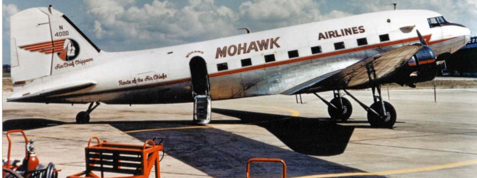
The venerable Douglas DC-3/C-47, represented here by Mohawk Airlines' DC-3-178, NC400D, c/n 1556, was popular during the 1950s with local service airlines because of their ready availability, passenger capacity and low operating costs. (Photo from the AAHS archives, AAHS-P006034)
