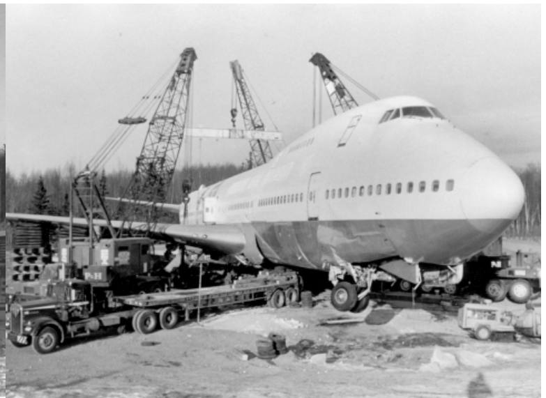
JAL 8122's severe chin and nose landing gear damage is seen here as the plane is slowly hoisted into the air. Airbags support the wings while the engines appear to have been removed. (JAL photo)
