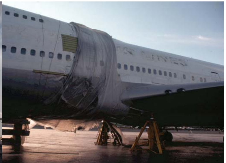
The large fuselage crack extending on both sides of the spine is protected from rain and snow until the AOG Team arrives. Heavy support jacks prevent 8122 from shifting during high winds. (Photo by the author)
