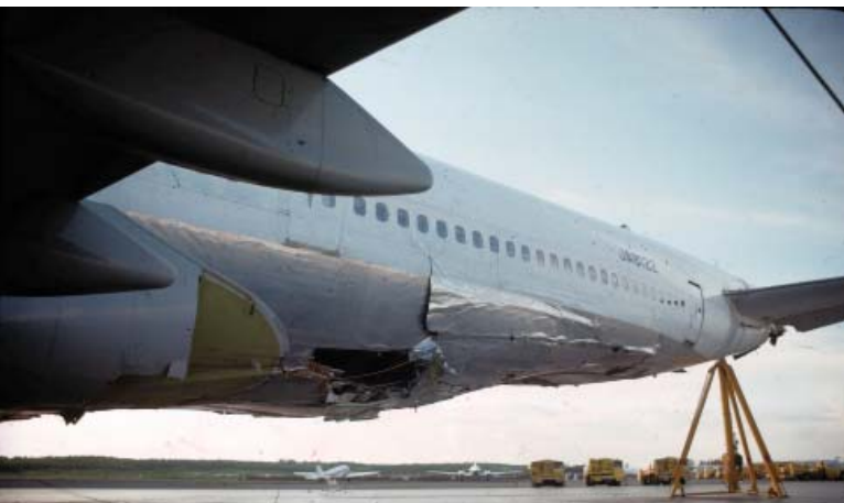
Damage to the lower aft fuselage is observed in this photo and tail stand to support the tail from shifting during further high winds. (Photo by the author)
