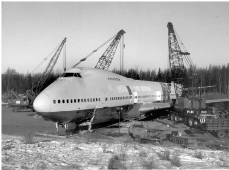
With its airliner name, logo and registration number obliterated and now representing Nobody Airlines, the JAL 747-200B has its fin-rudder removed. Lower chine crack and one just ahead of the wing-root right up to a side exit door is seen in this photo. (JAL photo)
