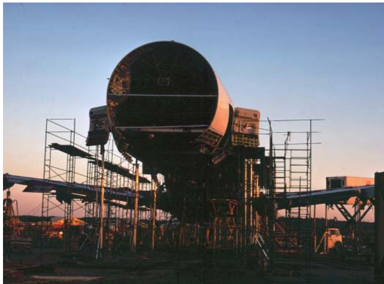
The AOG Team at work. Cranes have removed the rear fuselage and tail assembly to facilitate major repairs. Forward fuselage scaffolding is seen on each side of the giant mid-fuselage crack. (Photo by the author)
