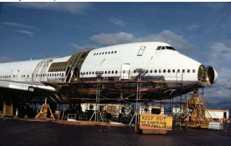
Several workers are seen in this photo taken weeks later showing the new replacement formers, stringers and skins painted zinc-chromate yellow. Plenty of lighting was positioned where necessary aiding the AOG night crew in their work. (Photo by the author)
