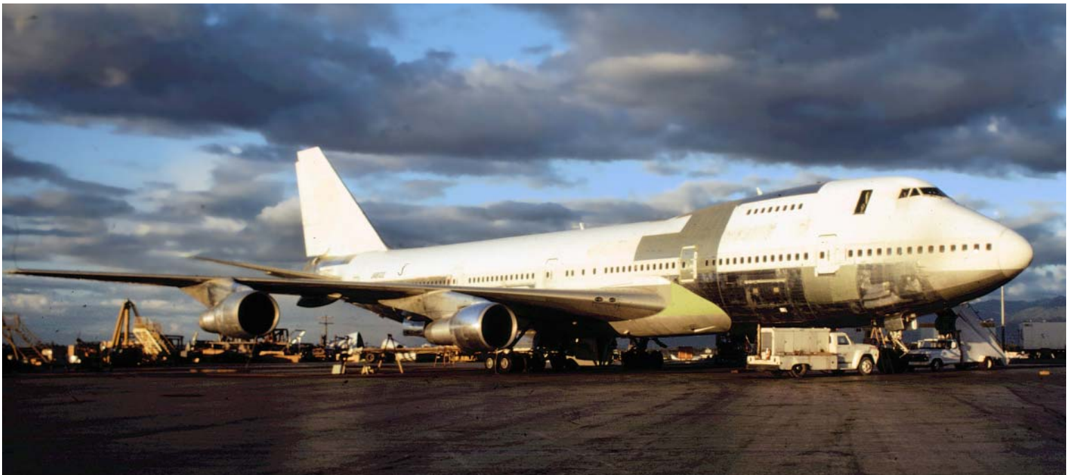
JAL8122 is now complete along with four newly mounted 50,000-pound thrust P&W JT9D-7FW turbofans. Numerous details are being attended to before the newly rebuilt 747 makes its initial test flight around Cook Inlet bordering the west end of Anchorage International Airport. (Photo by the author)
