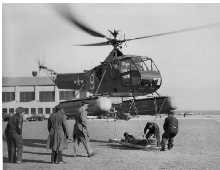
Experimental scoop to recover people in the water. Erickson rode in this device on a cold day as Graham flew. The extreme chill Erickson experienced during that one demonstration called for another option to recover people from the water. That pressure put the force behind the development of the hoist. (Photo from the author's collection)
