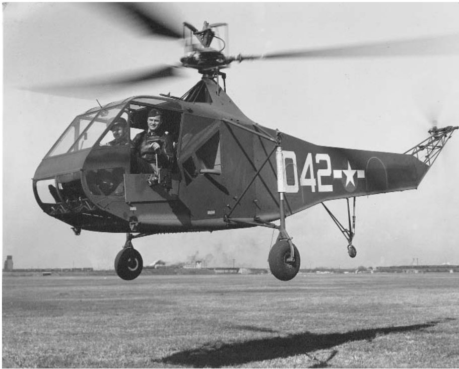
Graham, as the navy's first helicopter test pilot, flew a camera-rigged HNS to travel alongside a landing Grumman F7F Tigercat as it was being trapped in the aircraft carrier arresting gear located on navy's Muston Field, Pennsylvania. Engines were tearing loose from the airframe of the twin-engine fighter aircraft when being stopped by the arresting gear. The helicopter-mounted camera recorded the occurrences for later engineering study. (Photo from the author's collection)
