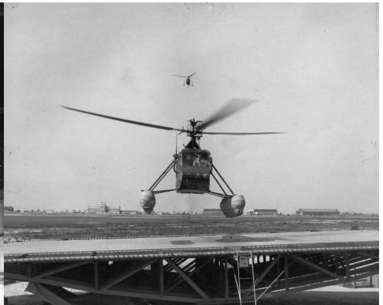
Left: The synthetic helicopter trainer developed by Erickson and Graham was scrapped before it could be put into instructional use. Above: HNS-1 landing on moving platform, Mal de Mer , the simulated ship landing deck on the field at Floyd Bennett Field. This platform mimicked the pitching deck of a ship in the open sea, and was also scrapped following the war. (Photos from the author's collection)
