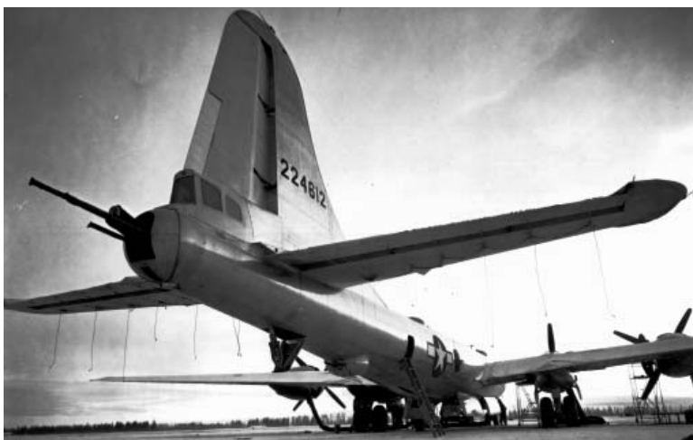
B-29 Klondike Kutey's rear armament of two .50 caliber machine guns and one 20 mm cannon was operated by a tail gunner inside a pressurized tail gun station. The B-29 CWTD report does not mention whether the guns were tested in sub-zero temperatures or not. (USAAF photo from the author's collection)
