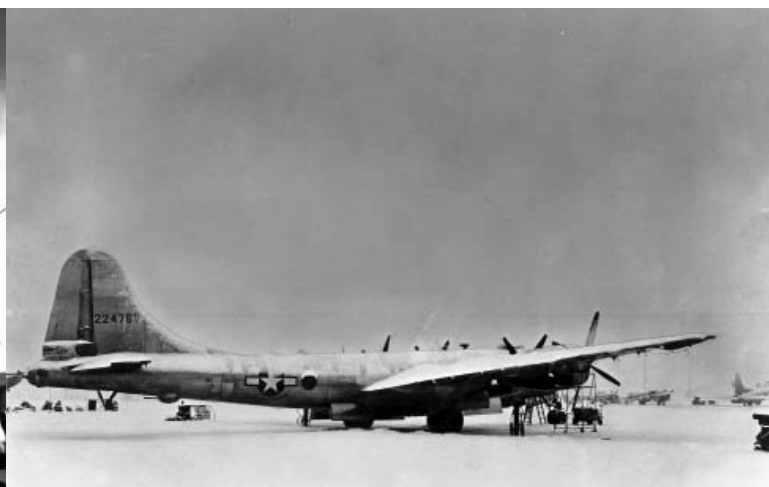
B-29 Amiable Amazon undergoes either maintenance or preflight check with a Jeep Heater off the nose. Large wing covers prevent frost buildup that takes hours to remove. A CWTD test B-17 and two P-38s are seen in front of the nose. (USAAF photo from the author's collection)
