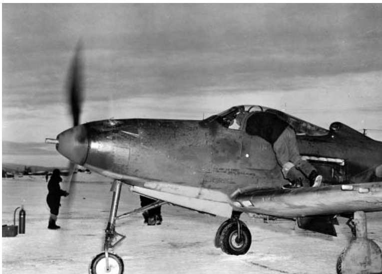
Lend-lease Bell P-39L-1-BE, 42,4673, runup test performed outdoors also displays the very delicate nose landing gear. The Russians performed field-modifications to strengthen them after delivery to the front lines. (Photo from the author's collection)
