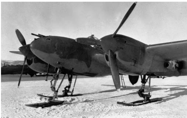
Lockheed P-38L with fabricated skis tested on several fighters assigned to the CWTD. (USAAF photo from the author's collection)
