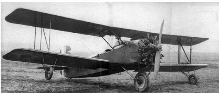
TA-5: Slightly larger TA-3 with larger engine modified for Engineering Division tests of single-wheel landing gear. YOM – 1923. Design: 2-place, open cockpit, biplane. Population: 1.
