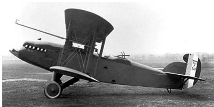
XO-3: Unknown D-W with some confusion about this aircraft. May have been initially designed by D-W but was built by Wright Aeronautical after GM dissolved the company in 1923. YOM – 1924. Design: 2-place, open cockpit, biplane. Population: 1.
