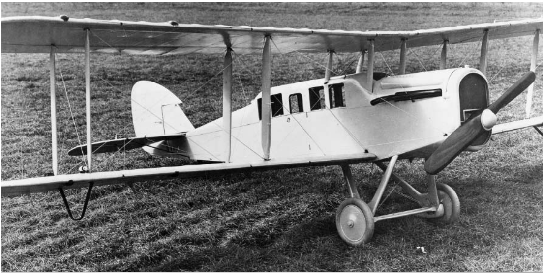
Left and Above: The KT Cabin Cruiser was a DH-4 derivative seating four in an enclosed cabin. (Photos courtesy of Special Collections and Archives, Wright State University, MS152-209, MS152-211)
