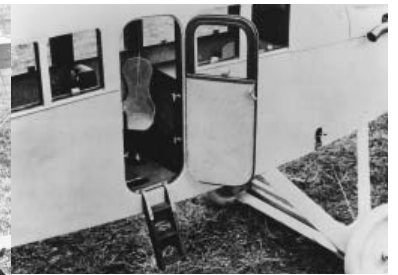
Left and Above: The KT Cabin Cruiser was a DH-4 derivative seating four in an enclosed cabin. (Photos courtesy of Special Collections and Archives, Wright State University, MS152-209, MS152-211)
