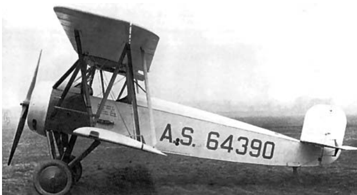
TA-3: Trainer based on the Chummy with side-by-side seating. YOM – 1923. Design: 2-place, open cockpit, biplane. Population: 13.
