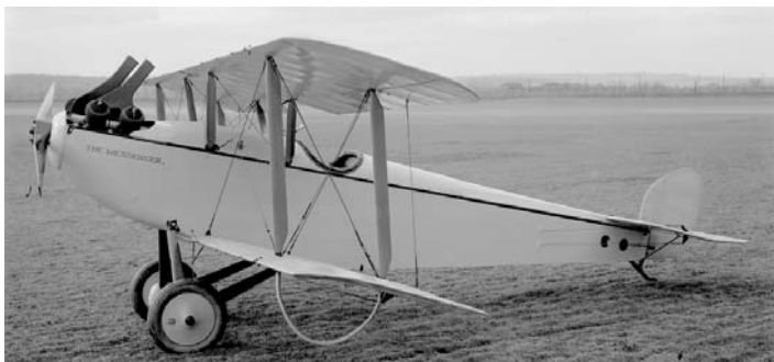
T-4 Messenger: Developed as an engine test-bed for the Kettering "Bug." YOM – 1918. Design: 1-place, open cockpit, biplane. Population: 1.
