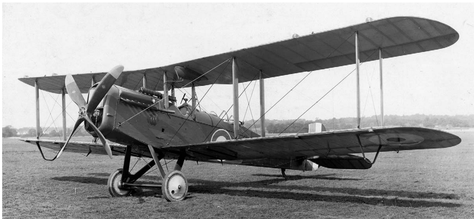
The DH-4 was based on a de Havilland design, modified to access a heavier, more powerful Liberty engine. Dayton-Wright would build over 80 percent of all the 3,800-plus DH-4s that were built during WWI. (USAAC photo from the author's collection)
