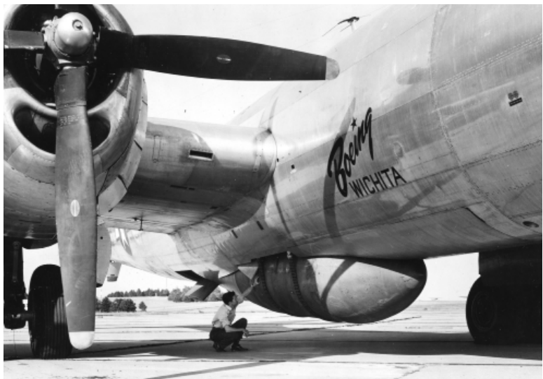
The largest conventional bomb ever dropped by an aircraft, the variously described 42,000, 43,000 or 44,000 lb bomb is seen here loaded on a specially modified B-29A, 44-6223. This aircraft would make six inert test drops over Muroc (Edwards) AFB in March 1948. Designed for the B-36, only two would ever be dropped from one - both from the same plane on the same flight. The B-36 flew a 2,900 mile round trip flight to Muroc from Carswell AFB, Ft. Worth, Tex., dropping the two inert bombs on a Muroc bomb range. (USAF photo from the AAHS archives)
