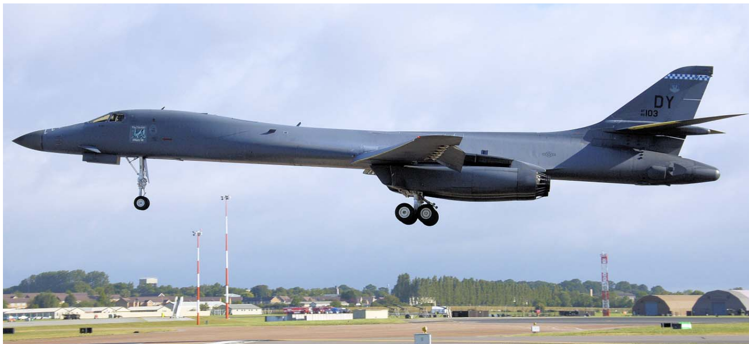
Rockwell's B-1B Lancer replaced General Dynamics FB-111s. Originally designed for a high-altitude high-speed penetration role, the B Models were reconfigured for low-level penetration. (Photo by Adrian Pingstone from the AAHS archives)
