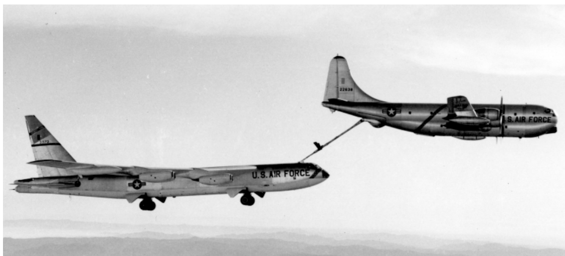
SAC operated a large fleet of tanker aircraft that over the years included KB-29s, KB-50s, KC-97s, KC-135s and KC-10s. Shown here is a B-52B receiving fuel from a KC-97G. (USAF photo from the AAHS archives)
