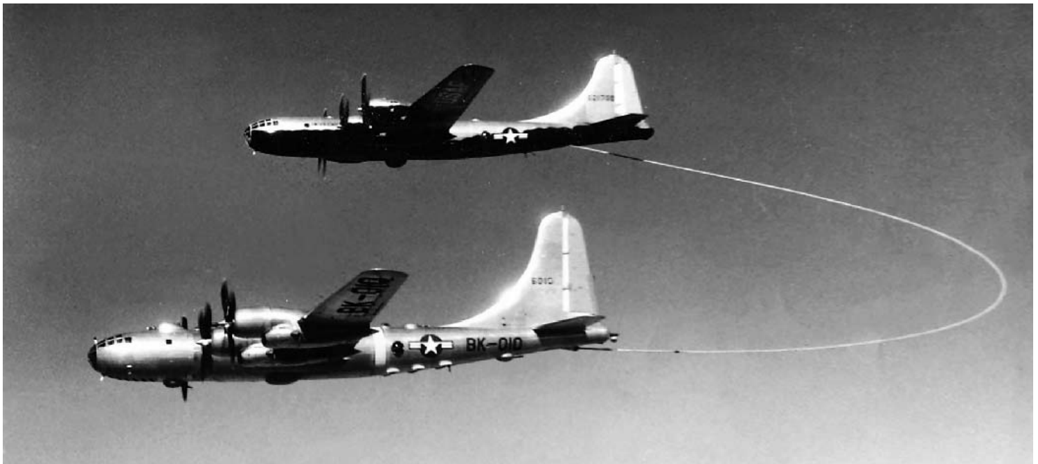
The B-50 "Lucky Lady II" refuels from a KB-29M during the 1949 round-the-world demonstration flight. The extent of the looped bight of refueling hose is clearly apparent. (USAF)
