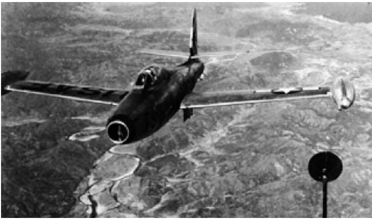
An F-84E prepares to hook up to the drogue for refueling. The probe is visible just inboard of the of the left wing tank nose. (USAF)
