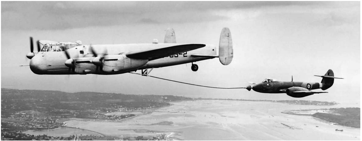
A Lancaster tanker refuels the Gloster Meteor fighter during a 1949 record-setting flight over southern England, using the probe and drogue method. (FRL)
