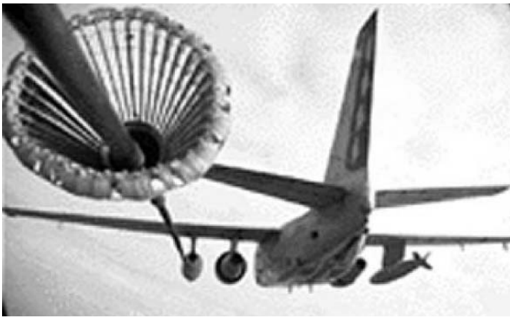
The pilot's view of the drogue just at contact. (USN)
