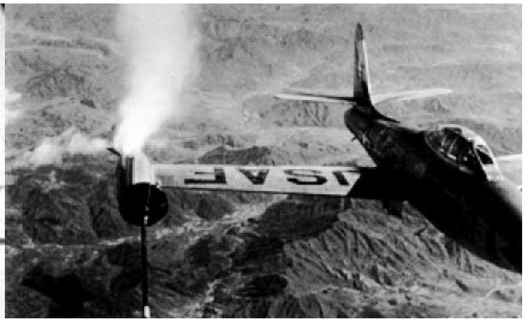
An F-84 refuels its tip tank over Korea, using the probe and drogue method. (USAF)
