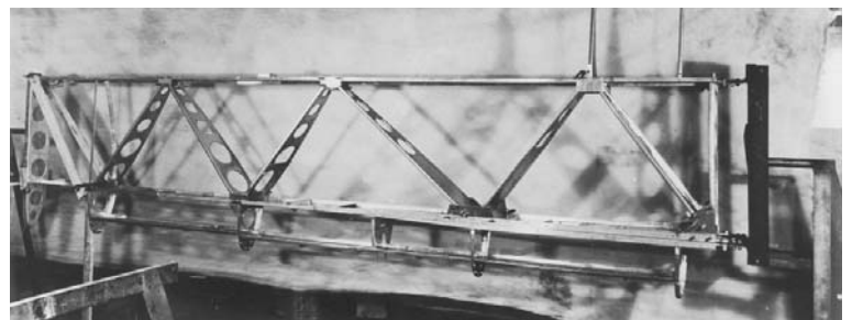
A view of the internal structure of Model 55's wing showing the diagonal rib arrangement that kept the part's count to a minimum. The wing ribs, nose and tip ribs and spars were all identical in both wing panels. Not counting the skin each wing panel consisted of only 19 parts. (Bendix photo No. 26142)
