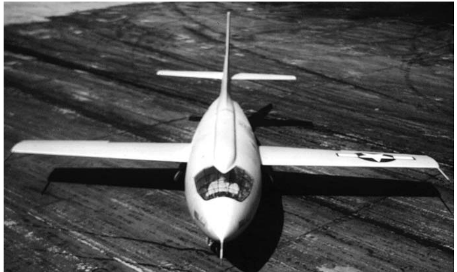
Overall design parameters of XS-1 are noted in this photograph displaying the ogive nose, bullet-shaped fuselage and straight wing layout. (Tim Whetstone, Lawrence D. Bell Aviation Museum)
