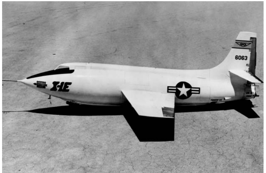
Bell X-1E number 2 X-1 (46-063) modified for high-speed flight. During its final flight on October 8, 1957, X-1E attained the quite impressive speed of Mach 2.24, a high achievement for mid-1940s technology and straight wings. (Ira G. Ross Aerospace Museum collection)
