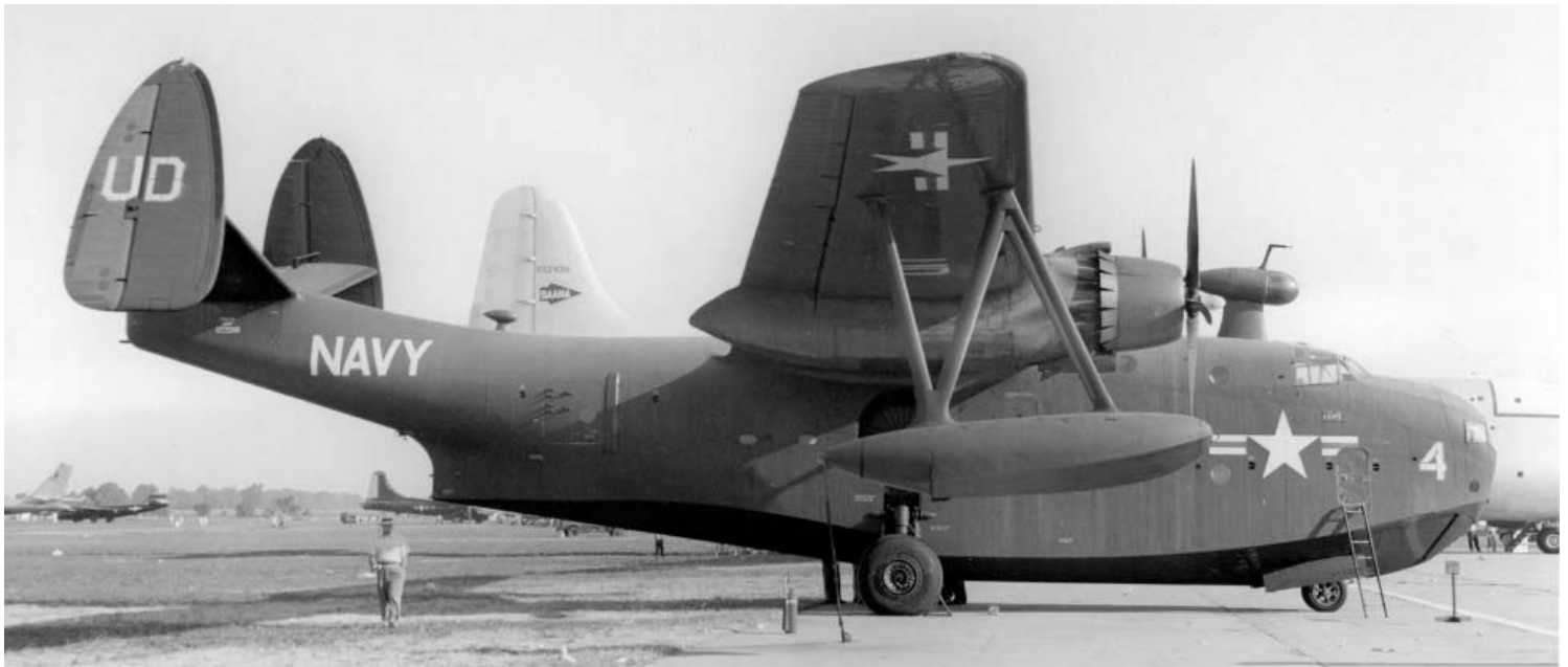
VP-203 was assigned Martin PBM-3s that were similar to this PBM-5A, BuNo 122081. The primary difference being that the -3s were equipped with Wright R-2600 Cyclone engines that produced 200 to 400 less horsepower per engine that the Pratt & Whitney R-2800s on the -5s. (Photo from the Al Hansen collection, AAHS-P000542)
