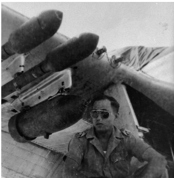
Primary armament for the RNEIAF P-51s in addition to the 50 caliber machine guns included 40 and 70 lb. British rockets and up to 500 lb. bombs. Here we see Ron van Beers' aircraft equipped with six 70 lb. rockets and what appear to be two 500 lb. bombs.
