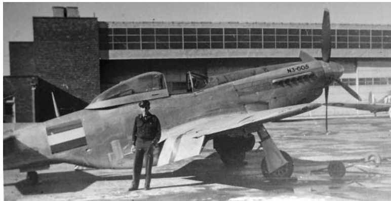
Photo of N3-605 taken in Canberra, Australia, in 1945. This is a P-51K with a "Dallas hood" and Aeroproducts propeller. The pilot is Arie de Jong. Registration number is black and four inches high on nose and tip of the rudder.
