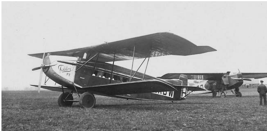
The F.V Biplane, with dorsal fin added and registered RR13 before its demonstration trip to Moscow in early June 1923. (Netherlands Fokker photo 623 from the Gert Blüm collection)
