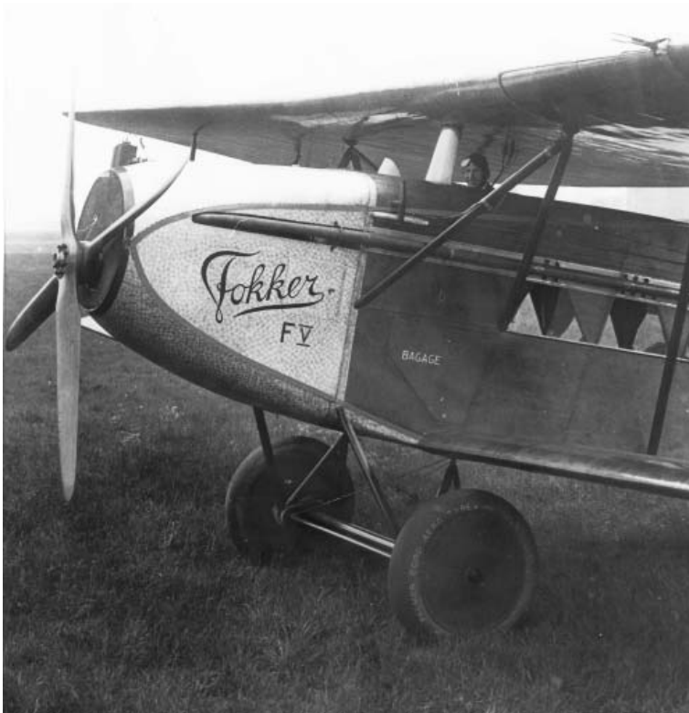
An altered pilot's windscreen is fitted and the aircraft's identity has at last been painted on the nose. (Netherlands Fokker photo 617 via Coen Smit)
