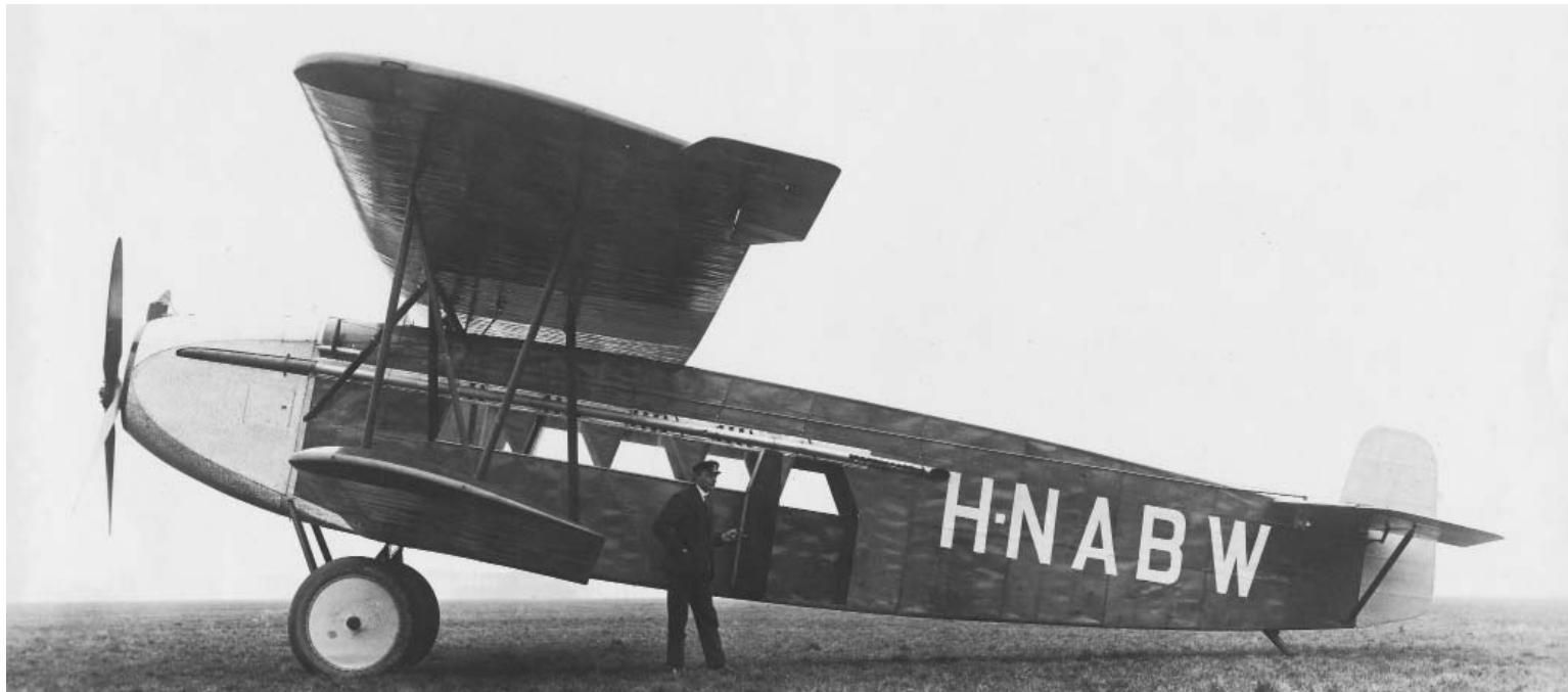
The F.V Biplane looks like it's ready to serve you. Note the newly introduced trapezium style rudder in this early 1923 photo. (Netherlands Fokker photo 521 from the Thijs Postma collection)
