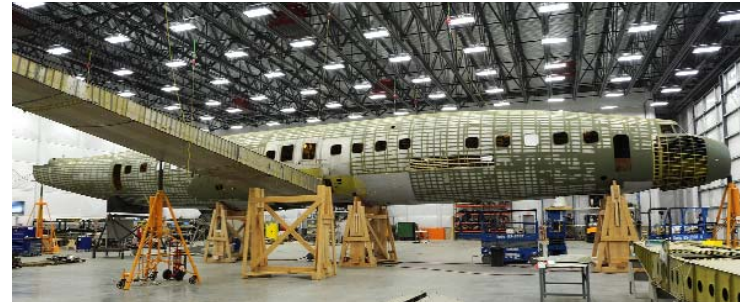
Starliner N7316C is being completely rebuilt by Lufthansa in what has to be the most ambitious Constellation restoration project of all times. The extent of the restoration is evident in this May 2009 photo taken at Auburn-Lewiston Airport, Maine. (Photo by the author)
