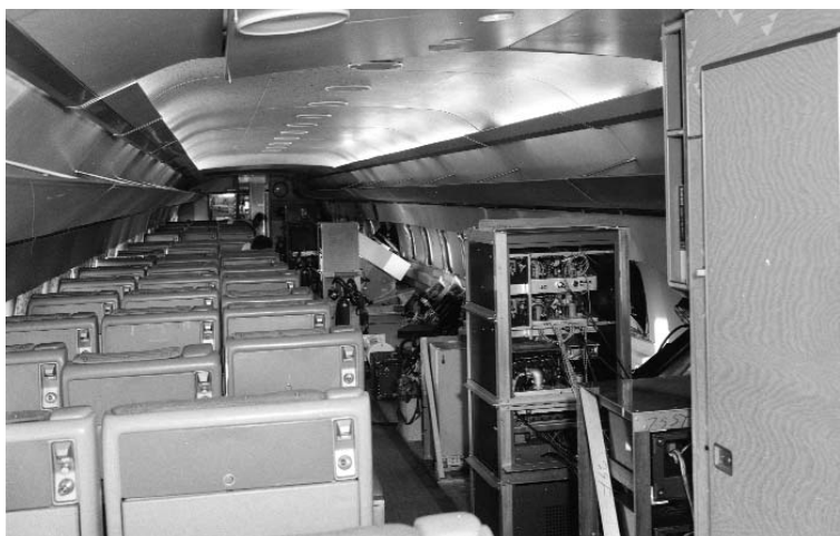
This view, looking forward, shows the modified main cabin with some seating on the port side and experiment sensors on the starboard. The experiments from Johns Hopkins and Service d'Aeronautic of Verrieres-Buisson, France in association with the University of Pittsburgh are in front of the seats. (DAC photo C 52652 from the author's collection)
