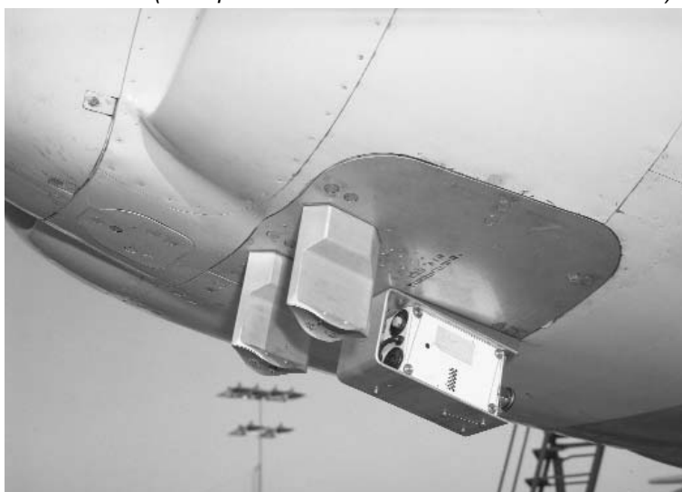
The two atmospheric aerosol collectors and the aft facing Benson-Lehner motion picture camera mounted on the left turbo compressor access door. (DAC photo C 52615 from the author's collection)
