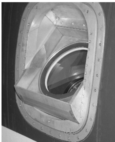
One of the articulated type observation windows is shown from the outside. These windows could be adjusted on a vertical axis. (DAC photo C 51625 from the author's collection)
