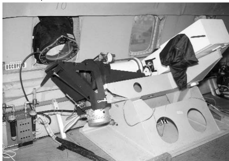
The Douglas Aircraft Company's spectrography experiment uses a flat panel placed at an angle equal to the altitude of the sun during the eclipse data gathering run. (DAC photo C 52654 from the author's collection)
