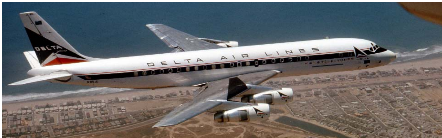
Flying above the Orange County coast, Delta DC-8-51 has been temporarily converted as a flying laboratory to gather data on a solar eclipse - the APEQS Project. Notice the anti-glare black area on the starboard wing and the variety of viewing windows on this side of N801E. (Photo from the author's collection)
