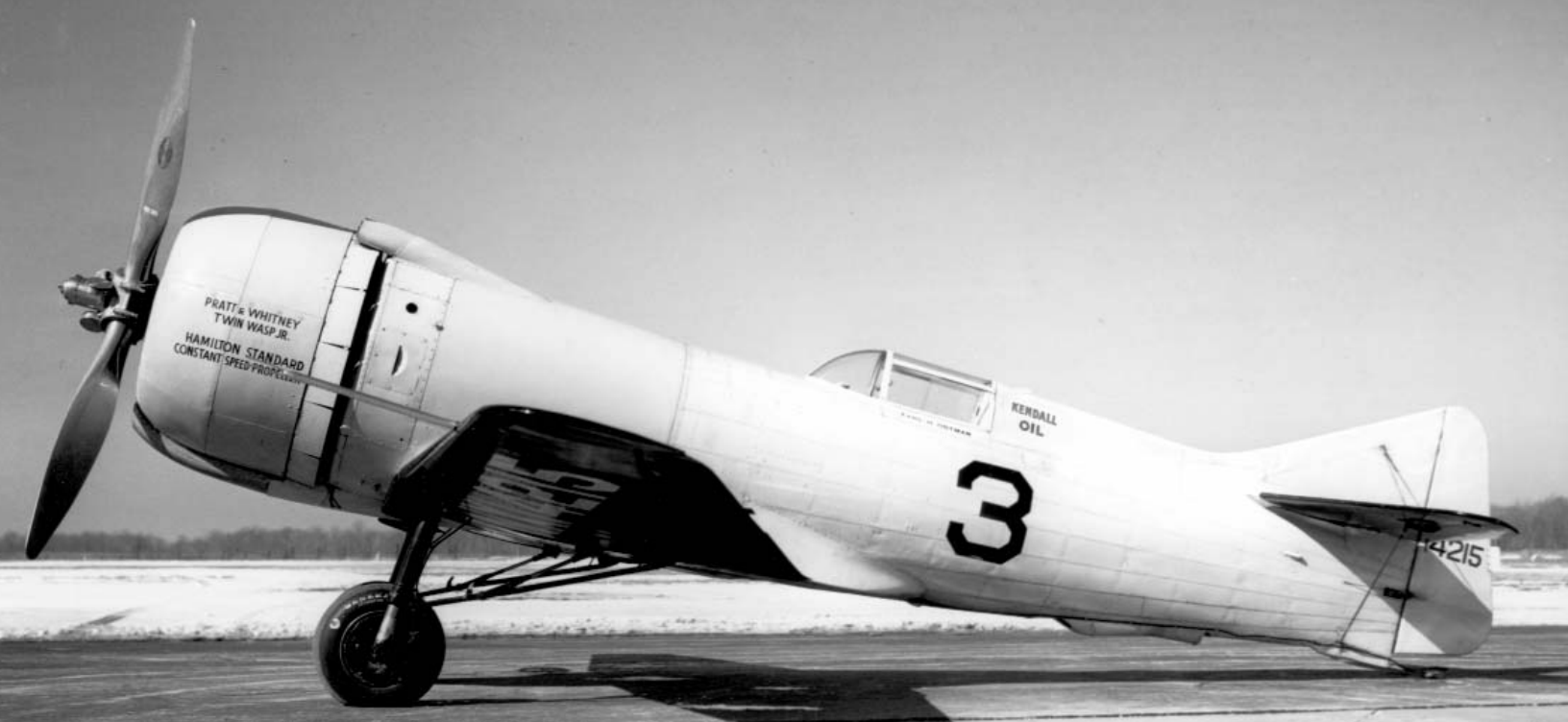
The Keith Rider R-3 was highly modified in 1937 by the new owners Marcoux and Bromberg. The modifications included a new wing, new engine and propeller, a new cowling and other changes. Ortman raced this aircraft at the NAR Thompson Trophy competition in 1936, 1937 and 1938 and finished second each time. (Photo by Bill Yager from the Strasser collection courtesy of Gerald Liang)
