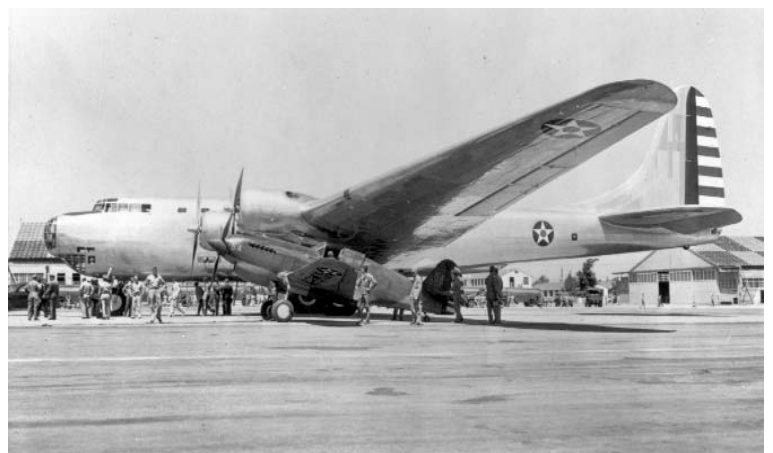
In 1938, the Douglas XB-19 began life as a design study - the XBLR-2 (experimental bomber - long range). The largest bomber built up to that time, development delays assured that the aircraft was essentially obsolete before its first flight in 1941. The aircraft was used for testing and cargo hauling until being scrapped in 1949.
