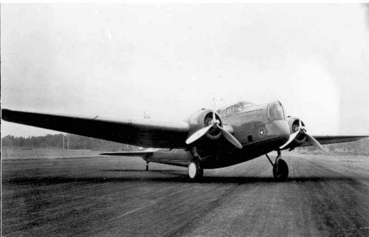
The Martin B-10 was the first all-metal monoplane bomber to go into regular use by the United States Army Air Corps, entering service in June 1934.
