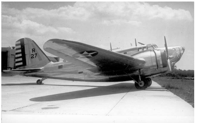
Between 1937 and 1939 the USAAC ordered 217 Douglas B-18As. B-18s would form the bulk of the bomber force in the late 1930s and early 1940s. Its poor defensive armament, and being underpowered, relegated it to second-line service by 1942.
