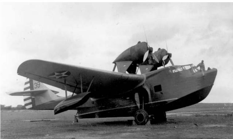
The Douglas YB-11 started life as the YOA-5 and was as an amphibious reconnaissance-bomber, intended to act as navigation leaders and rescue aircraft for formations of conventional bombers. Only one was built, but it was used to set two world distance records for amphibians.
