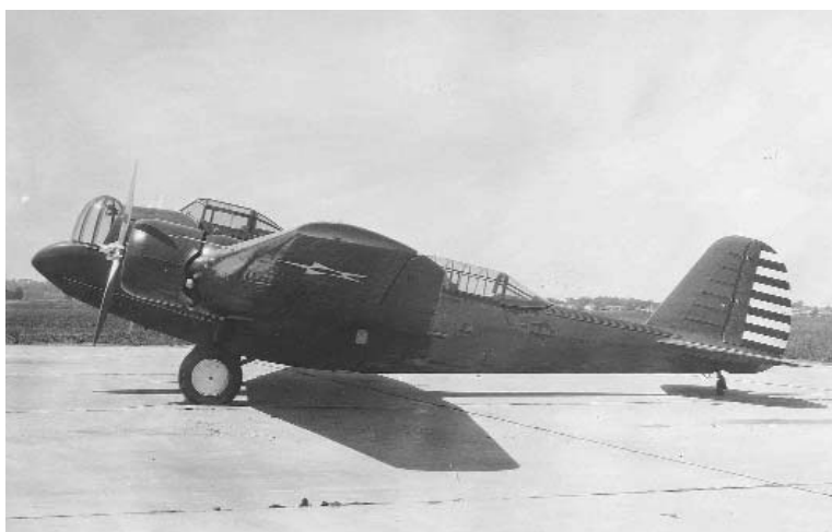
The Martin XB-14 differed from the B-10 only in its powerplant that was a P&W YR-1830-9 Twin Wasp. The B-10 and its variants formed the backbone of the U.S. Army first-line bomber force during the mid-1930s.
