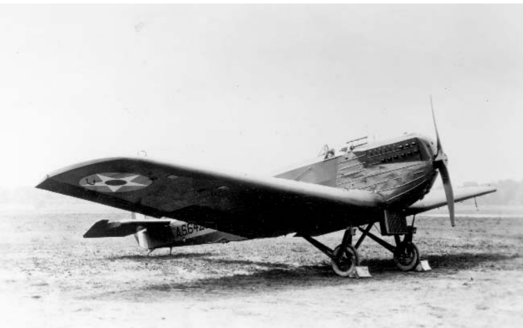
The 1923 Gallaudet DB-1B (Day Bomber designation) was the first attempt to build a monoplane bomber for the U.S. Army. It proved to be about 10 years ahead of its time. Only two were built and only the DB-1B actually flew.
