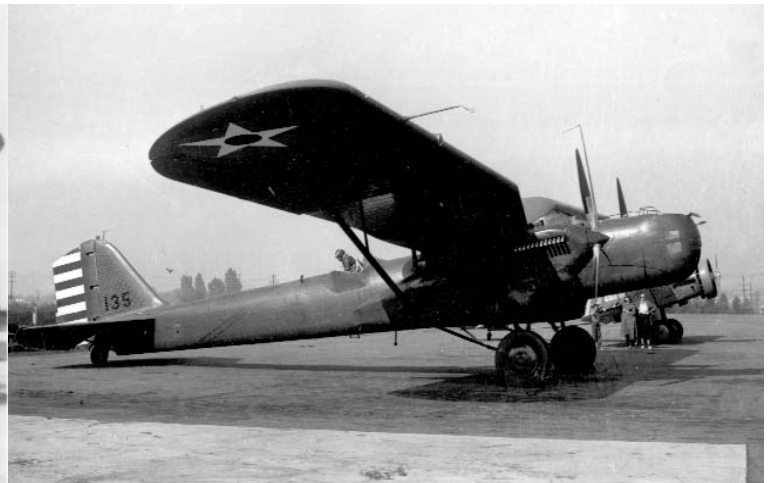
Douglas B-7 was also offered as the Y10-35; failed to merit a production contract in either category. During a tragic few months in 1934, it ended its career flying the air mail. Top speed 182 mph.
