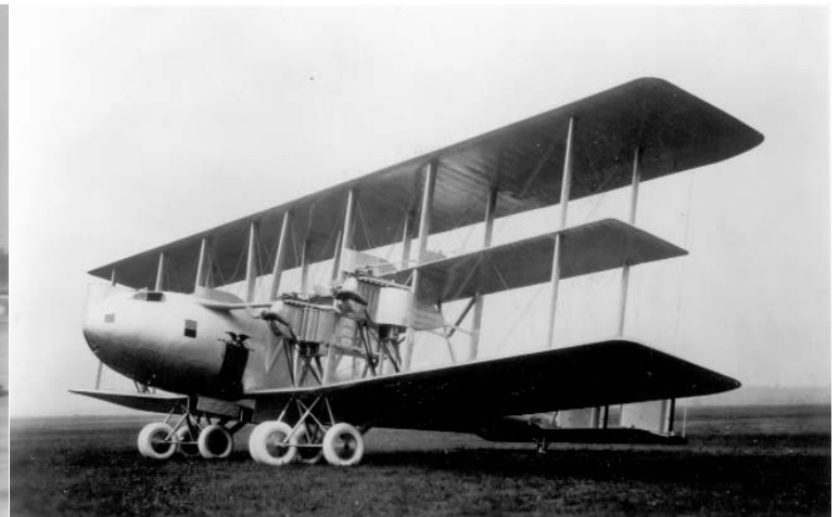
The Wittenman-Lewis NBL-1 (night bomber long distance) was a six-engine, three-wing disappointment. With full fuel and bombs it had a range of 170 miles, half the distance of the smaller NBS-1. This was the only one built.
