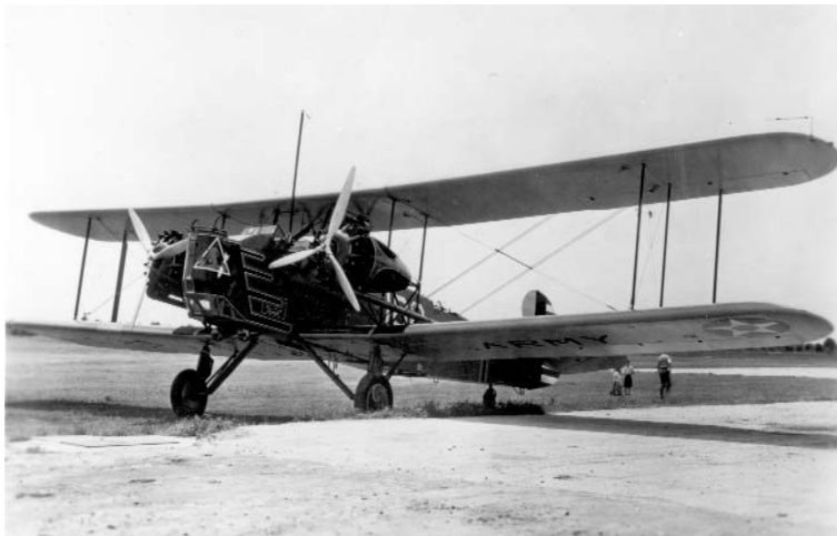
The 1929 Keystone LB-6 was a simple improvement to the LB-5 featuring a modified tail and lengthened fuselage. Variants of the design (B-6A) would be the last biplane bomber purchased by the Army in 1932. Its performance was only slightly better than the Martin NBS-1 of 1921.
