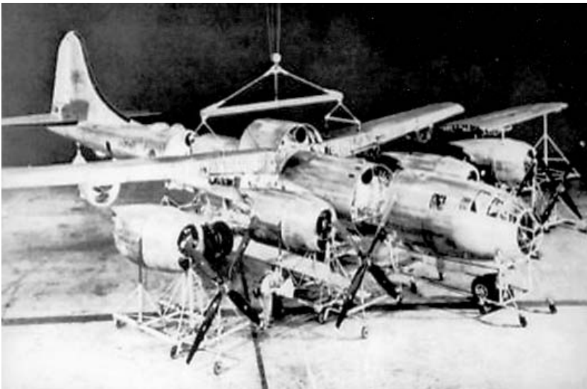
A Boeing Company PR photo of an exploded B-29 demonstrating the component structure. Powered by four Wright R-3350s the bomber was truly an innovative air weapon, a true superfortress, as it was the first heavy bomber produced to include a tricycle landing gear, autopilot, tandem bomb bays, pressurized crew compartments, and remote central fire control. It was the forerunner of today's "systems" aircraft. (Boeing via Pima ASM)
