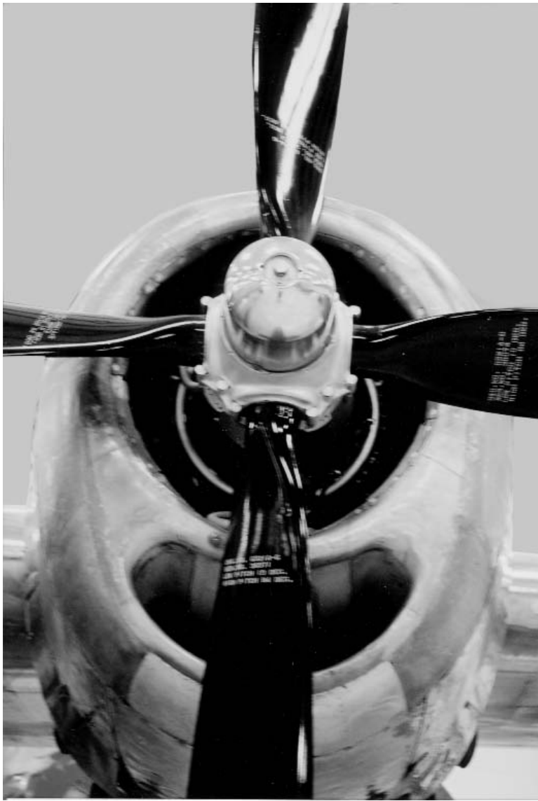
The R-3350 mounted Hamilton-Standard (a division of United Aircraft Corp.) 16.67 foot steel four-bladed, hollow, electric, hydromatic, constant speed, full-feathering propellers, which were the largest fitted to an American production aircraft. (Author/Pima ASM)
