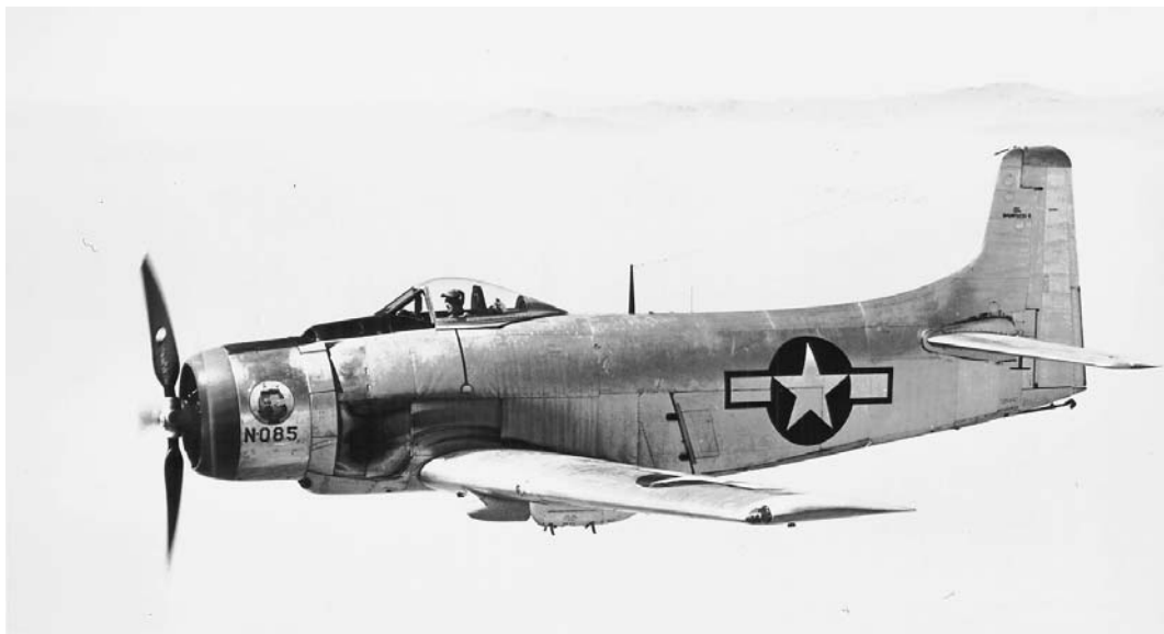
The Douglas XBT2D-1, BuNo 09085. This design would evolve into the ubiquitous A-1 Skyraider powered by the R-3350 and proved itself an effective propeller-driven jack-of-all-trades in the jet age aerial warfare over Korea and Vietnam. (USAAF)
