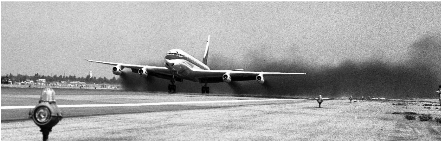
The early JT3 engines generated a large amount of smoke on takeoff due to water/alcohol injection. The replacement of these engines by JT4As allowed the elimination of this cooling system resulting in a weight saving of around 5,000 lbs. (Photo from the author's collection)
