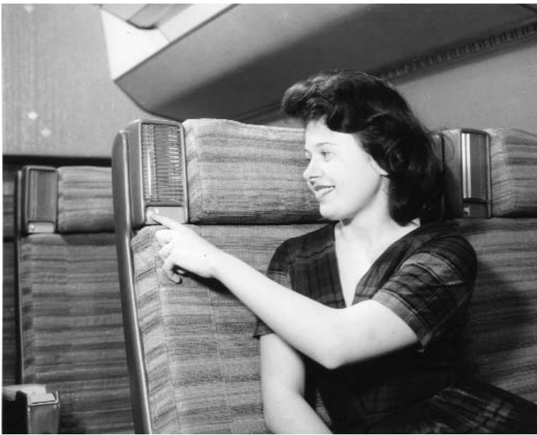
Passenger seating included individual stewardess call buttons as seen being demonstrated here in the first class section. (Douglas photo EST-C-1598B)
