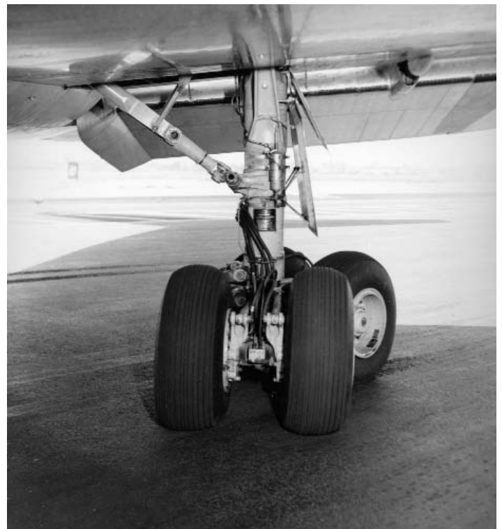
The DC-8’s main gear bogies were designed to allow them to swivel, facilitating tight turns without scrubbing the tires. (Douglas photo C-8-2323-2)
