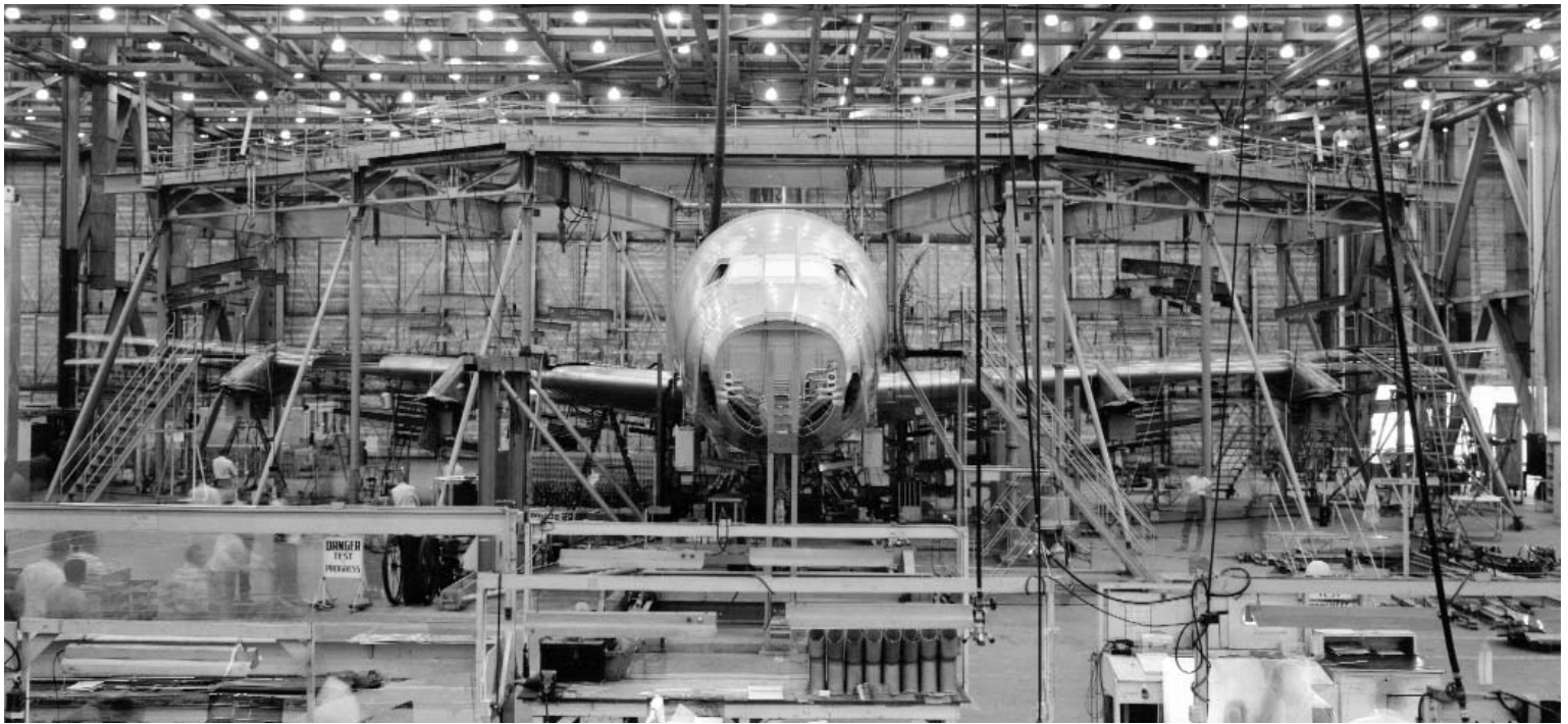
Ship Two, N8018D, undergoing static testing at the Long Beach facility. (Douglas photo MSN 45278)
