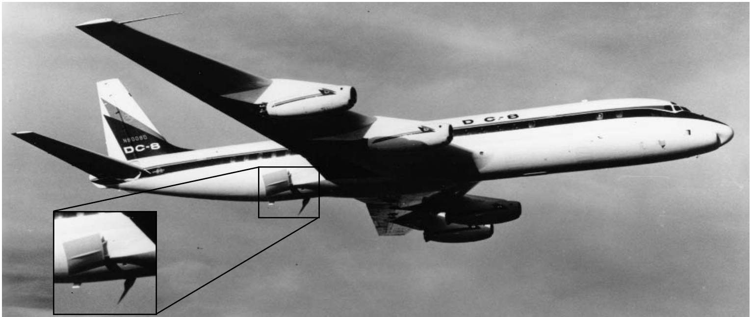
Ship One was equipped with speed brakes which were eliminated because they were ineffective. (Douglas photo A811-7-9)
