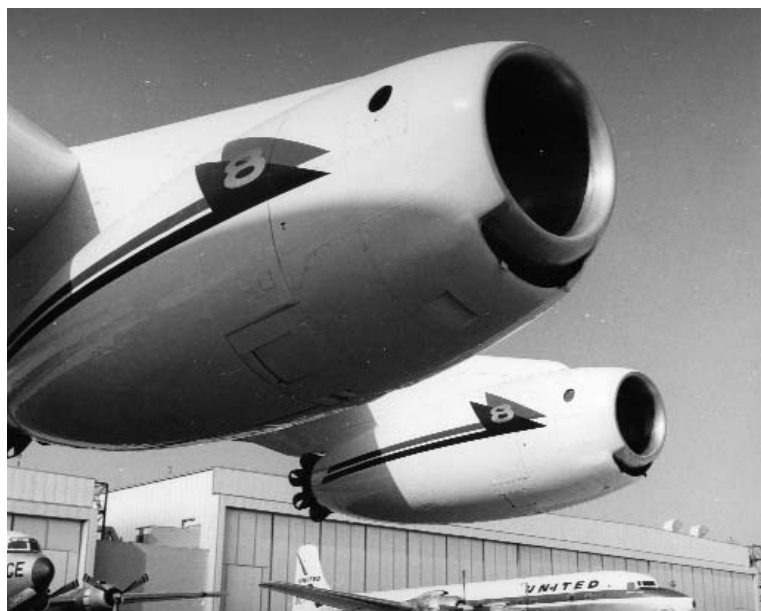
Examination of the engine nacelles on Ship 1 (N8008D) reveals the lack of thrust reversers. These were not added until Ship 3 and subsequently installed on all airframes. (Douglas photo SM255626)
