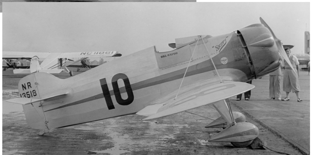
The Rasmussen "Skippy" racer, NR13518, race no. 10, was powered by a 5-cylinder 190 cu. in., 65-hp engine. The plane, flown by Willis Kysor, won a second and a third place in the 200 cu.in. events.
