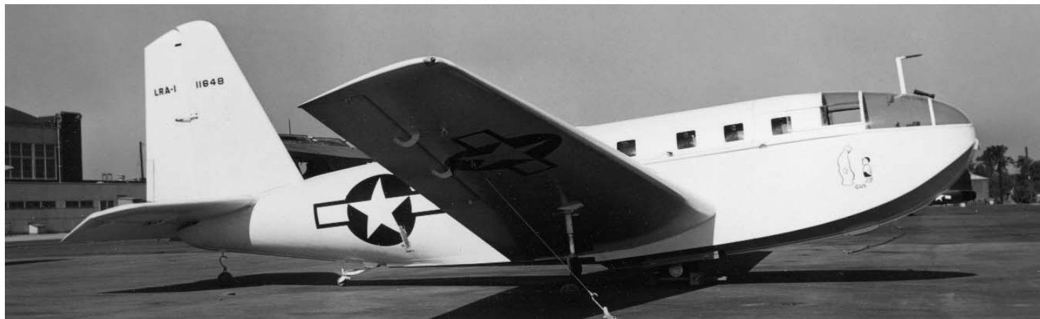
The second Invader prototype shows a further evolution in the canopy design. Although a true tricycle undercarriage was called for, a compromise is evident in the wheels added to the tail and wing skids. (National Soaring Museum)
