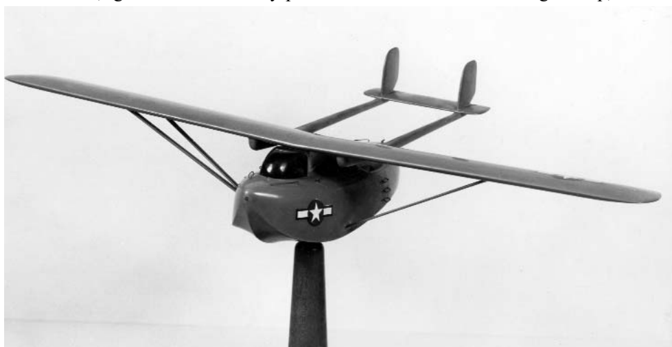
With uncertainty as to the suitability of the float-wing concept, other ideas were suggested. This high-wing design, possibly the 12-place Allied XLR2A-1, apparently gained stability on water simply from the width of the hull since it lacked outrigger floats. (Jay Miller collection)
