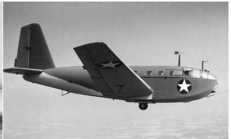
At this instance in a test flight, the XLRA-1 has its landing gear extended and is in a low tow position. Pitot probe and sideslip vane are well above the aircraft to avoid water spray impact. (National Soaring Museum)
