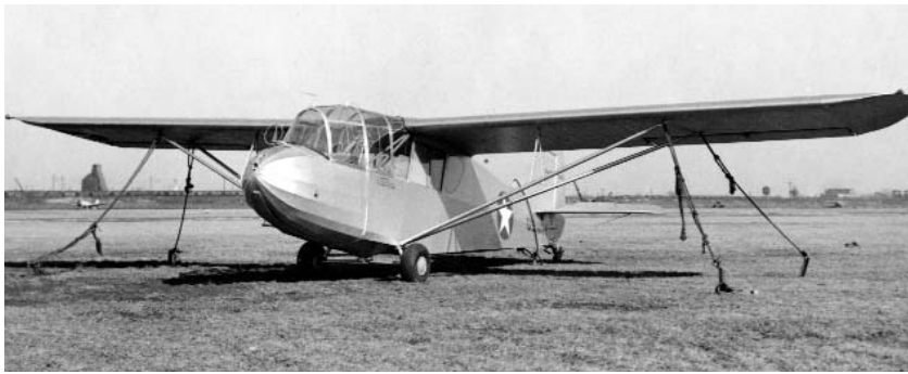
The Aeronca LNR-1 was another three-place trainer from the Army where it was known as the TG-5 and developed from the L-3 light plane. Three of these were evaluated in late 1942 to fill the Marine training role. (National Soaring Museum)
