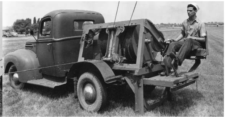
To support efficient glider launch for Marine pilot training, the Navy procured this Gar Wood truck-mounted winch. There was a throttle and speed control to pull a glider up to flying speed and then reel in the cable once released, or cut the line in an emergency. (National Soaring Museum)
