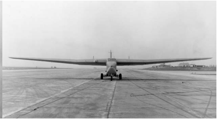
Unlike the troop transport gliders, the XLRN-1 showed no evidence of being intended for water operations, although this may have been merely an expedient for an initial design. This view emphasizes the thick wing with a leading edge bulge for a generator, and the cross-beam main undercarriage. (National Soaring Museum)
