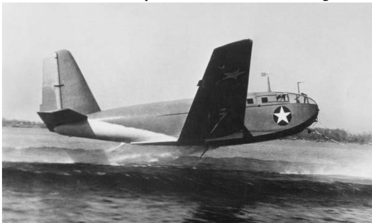
The initial example XLRA-1 lifts above the surface of the Delaware River during flight trials in 1943. The stepped hull and tow line attachment are evident. (National Soaring Museum)
