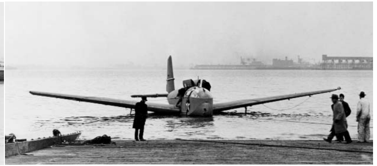
The XLRA-1 approaches the seaplane ramp at the Philadelphia Navy Yard following a test run on the water. The hatches on both sides appear to offer ready access to the interior. (Naval Aviation Archives)
