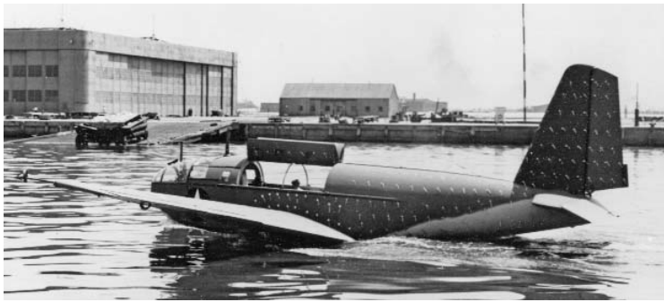
The first XLRA-1 prototype motors along at slow speed with its outboard motor during testing in 1943. Tufts are attached to the surface of the aircraft to enable visualization of airflow. (Naval Aviation Archives)
