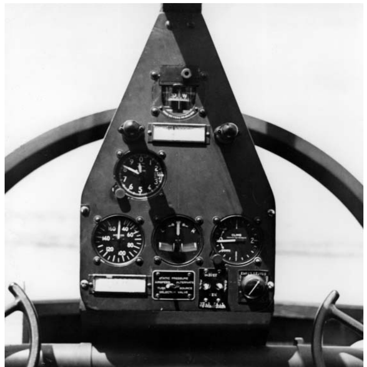
The spartan instrument panel of the XLRA-1 Invader is arranged in a vertical fashion and affords excellent vision forward. The dual control wheels are provided for the aircraft commander and second pilot. (Naval Aviation Archives)
