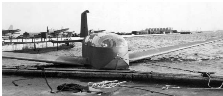
The Bristol XLRQ-1 is seen during water testing in Philadelphia in 1943. At this time, the glider lacked any wing root fairings for main undercarriage retraction. (National Soaring Museum)
