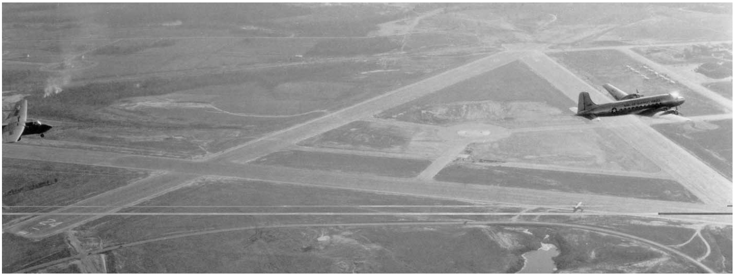
The great mass of the XLRN-1, at 36,000-lbs fully loaded, meant that only a 4-engine transport was suitable to tow it aloft at anything but nearly empty weight. A Douglas R5D-1 hauls the glider across the NAS Patuxent River backdrop. (National Soaring Museum)
