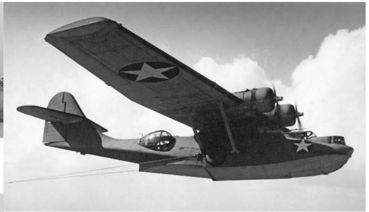
The NAF's PBY test support aircraft was given the nickname "Tugboat Annie" to reflect its new job. Note the nylon tow line attached to the fuselage at two points as a bridle. (National Soaring Museum)
