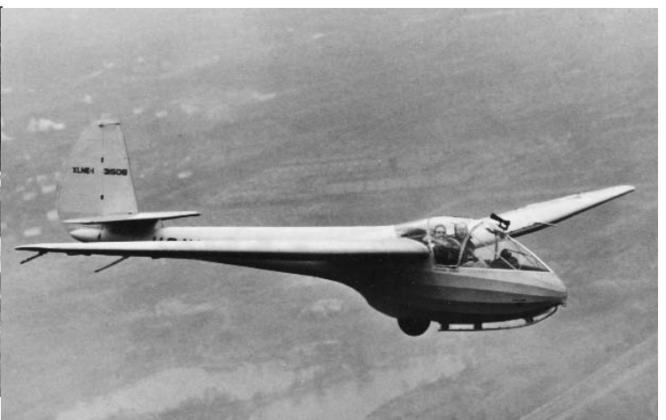
The prototype Pratt, Read XLNE-1 training glider (PRG-1 to the builders) is seen in flight, probably in spring 1942. The side-by-side seating was very unusual for the period. (National Soaring Museum)
