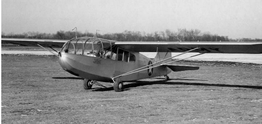
The third three-place trainer was bought in slightly larger numbers, but ended up being used mostly as bomb glider testbeds. The Taylorcraft LNT-1 was derived from the L-3 'Grasshopper' liaison aircraft and known to the Army as the TG-5. (National Archives)
