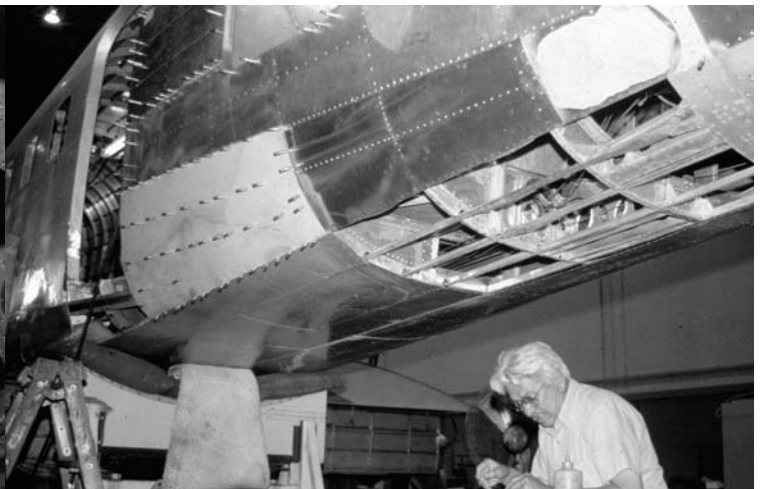
Replacing fuselage exterior skin that had been severely dented skin that had been damaged by the parachute lanyards during jumps by fire fighters at low altitudes into fire areas.
