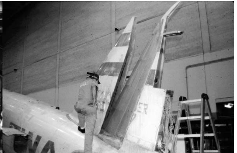
Removing the vertical fin leading edge for reconditioning. This was an add-on to overcome the lack of directional control after losing one engine on takeoff.
