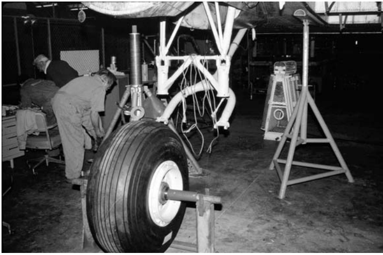
Assembly and installation of reconditioned landing gear components.
