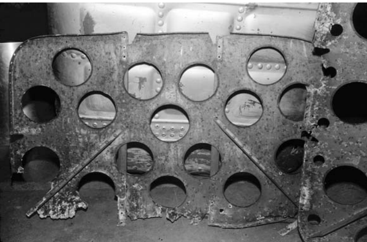
Photo showing condition of a fuel tank prior to reconditioning and rebuilding.
