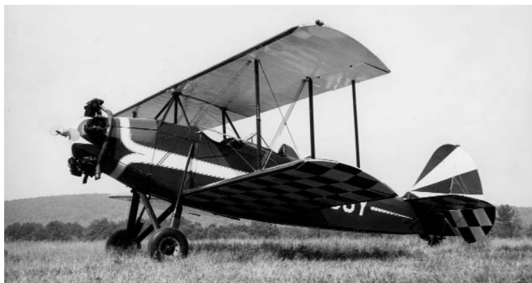
In later years s/n 26, NC753Y, B-8 Kitty Hawk was fitted with possibly an Aeronca vertical fin and rudder in North Carolina. It really spoiled the original looks of the B-8. (Photo from Wally Smith)
