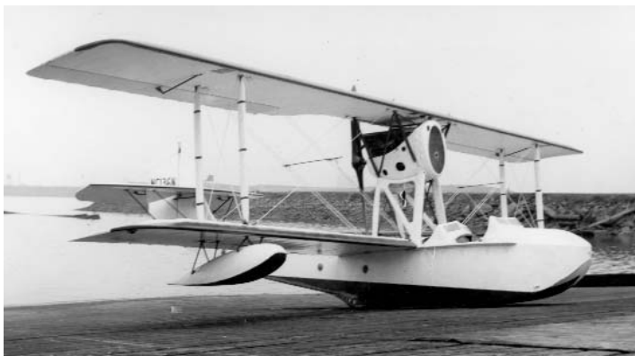
Evident here are the beautiful lines of Schreck flying boat, s/n 64, NC136N, powered by a Hisso 180-hp engine, at New Haven. The color of this craft is likely yellow with black bottom. (Photo from the Warren Shipp collection)
