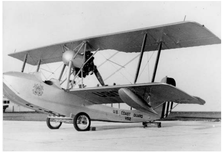
Another view of #152, with the Wright J-6-7 (R-760) 240-hp engine. The photo location is unknown. (United States Coast Guard photo from the author's collection)
