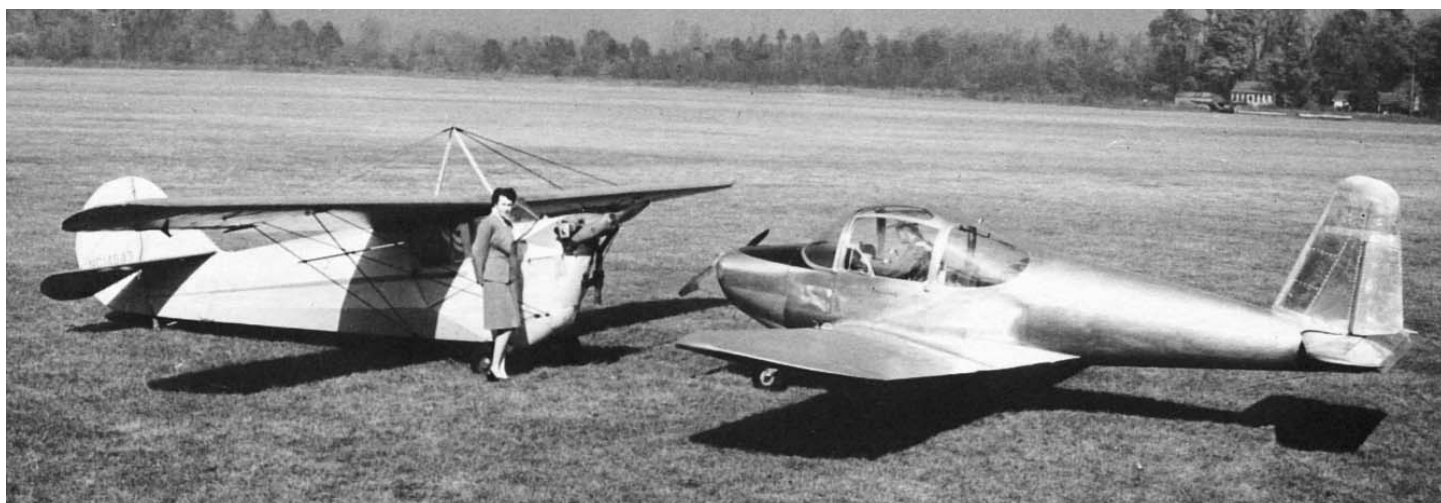
Aeronca's long design evolution stretched from the early "flying bathtub" C-3, (left) to the modern, aluminum, tricycle geared Chum (right). While the rest of general aviation headed towards the "modern" design -- Aeronca would wind up returning to basic design ideas of the C-3, eventually producing one of the most popular personal planes ever. (From Aeronca: A Photo History, by Hollenbaugh & Houser)
