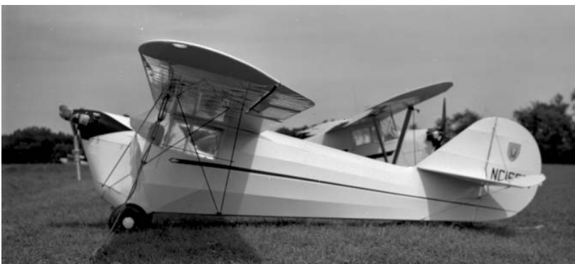
Late-1930s Aeronca C-3: adding windows, doors, and a bit less wintertime draft. The slightly reduced noise made instructing easier, long flights more tolerable. Notice the refined shape, with stringers rounding the formerly triangular fuselage. On top (blocked from view by the wing) are the twin kingposts and wires supporting the wing. (Photo by William Steeneck from the AAHS photo archives, #4644)
