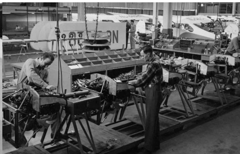
Mass production perfected in puddlejumper: Aeronca introduced the first automotive-factory-style mechanically moving assembly line in general aviation, using a chain on a track in the floor to continuously move fuselage airframes - tail-end-first - from first welds to final fabric covering, and out the door, at a record pace, producing an average of 30 planes a day - once building an astonishing 56 planes in a single day! (Photo from Hollenbaugh & Houser collection, via Brian Matz, Aerial Aspect Photo)
