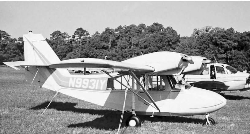
1963 Champion 402 Lancer, N9931Y, s/n 9, shows the complex gear and strut arrangement required to support the twin engine design. (Photo taken in 2003 at EAA Sun 'n' Fun by Timothy Aanerud)
