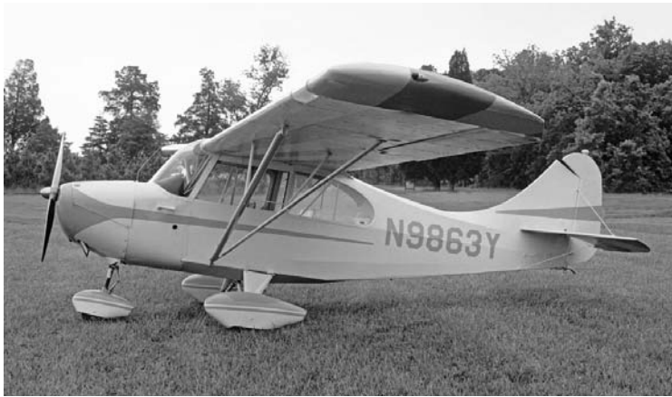
A tricycle Aeronca? Only one 7FC Tri-Traveler was built under the Aeronca name. It took Champion Aircraft to put a tandem Champ on tricycle wheels and sell them that way -- many of them -- in the rapidly changing trainer market of the 1950s, where touchy tailwheels were being replaced by safer, more popular tricycle gear. (Photo by Robert Burns)
