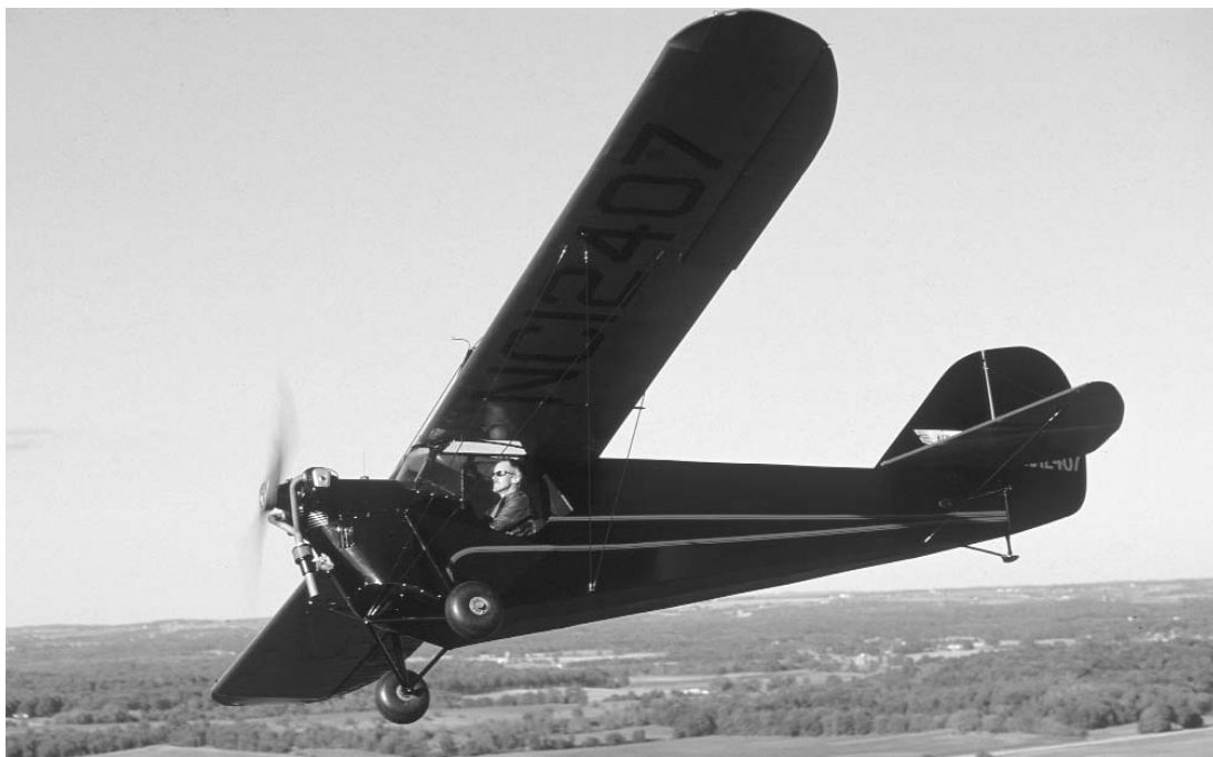
Jean Roche's own, personal 1931 Aeronca C-3. Two seats, 60-70 mph, gentle handling, mediocre visibility, and great fun on just pennies. It arrived as the cheapest brand-new trainer and sport plane in the world -- to own or operate -- except for its single-seat predecessor, the C-2. Roche fitted his with Edo 1070 floats -- and kept it until 1966. Here, in its element, it is piloted by Jim Hammond -- only its third owner in three-quarters of a century. (Photo by Jim Koepnick from the EAA Vintage Aircraft Association)
