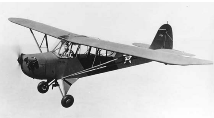
Aeronca L-3 Grasshopper: Whether flying out of tiny jungle clearings or launched from ships, Aeronca’s simple, practical, glass-enclosed “observation” plane brought exceptional utility to the war -- moving supplies to the front, and wounded to the rear, spotting for artillery and allowing field commanders easy observation of the entire battlefield. Over 1,200 were built. This one sports the “greenhouse” canopy for easy observing, and a wind-driven generator between the gear-legs, to power a radio. (U.S. Army photo from the Army Aviation History Web site)
