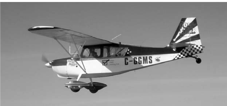
Showman Daryl Lowey's 1975 Bellanca-Champion Citabria 7KCAB, rated to +5 and -2 Gs with fuel and oil systems modified for inverted flight. (Photo courtesy of Daryl Lowey, www.livingskyaerobatics.com )
