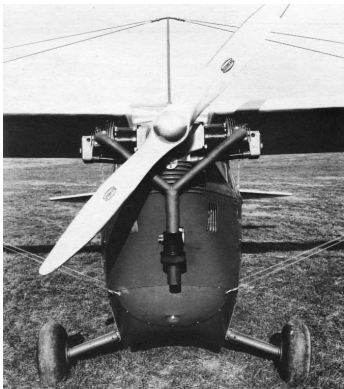
1937 Aeronca C-3, showing off the Aeronca E-113 engine, derived from the E-106, in turn crafted by Roy Poole and Robert Galloway from Morehouse's original, but quickly destroyed, design. Two-cylinder, four-stroke, single-ignition, Y-shaped exhaust, and a whopping 36 hp. In this later model, a single shock absorber is concealed inside the fuselage. Note the kingpin and wires holding the wing in place. (From Aeronca: A Photo History , by Hollenbaugh & Houser)
