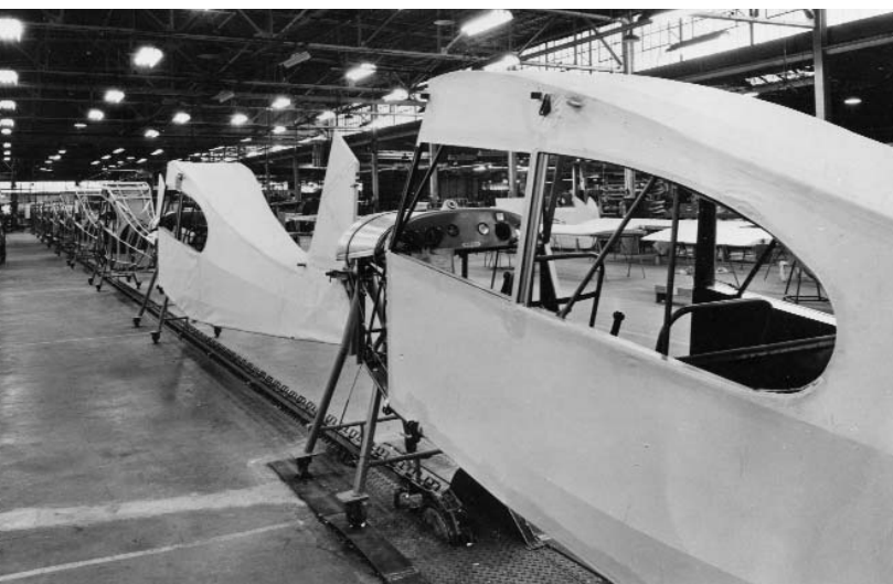
Mass production perfected in puddlejumper: Aeronca introduced the first automotive-factory-style mechanically moving assembly line in general aviation, using a chain on a track in the floor to continuously move fuselage airframes - tail-end-first - from first welds to final fabric covering, and out the door, at a record pace, producing an average of 30 planes a day - once building an astonishing 56 planes in a single day! (Photo from Hollenbaugh & Houser collection, via Brian Matz, Aerial Aspect Photo)
