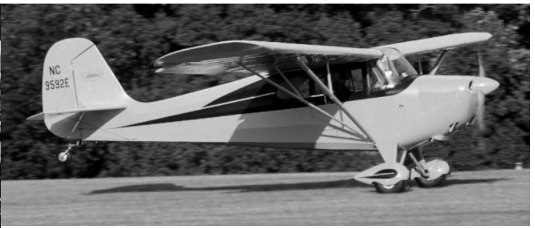
To meet preferences of personal flyers, Aeronca returned to the idea of the socialable side-by-side cruiser, with its 11AC Chief - capitalizing on Aeronca's popularity, dealer network, and the efficient matching of many of the 7AC's parts and much of its design. A lot of fun airplane on a little bit of money and engine, the postwar Chiefs were the last great gasp of two-seat, side-by-side, tube-and-fabric taildraggers -- soon to be outclassed by the faster all-metal Cessna 120/140, and by the emergence of the 4-seat "family sedan of the air." (Photo by Charles E. Stewart)
