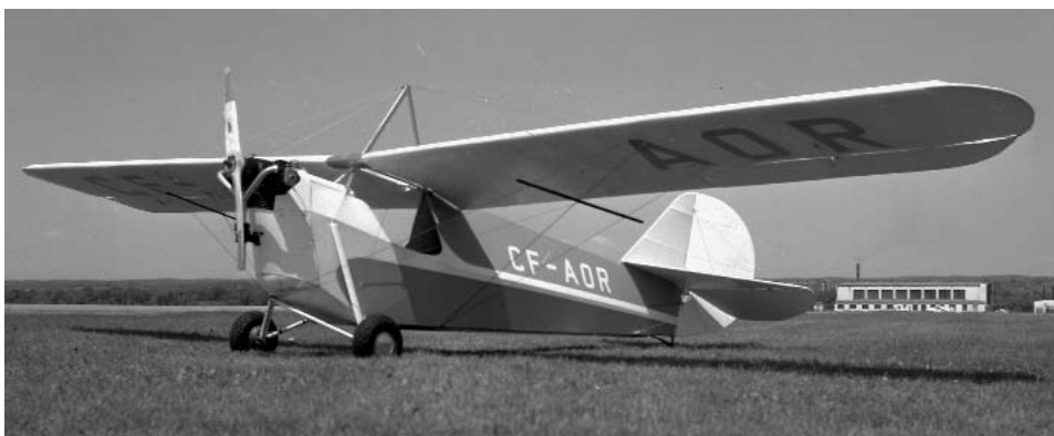
Aeronca C-2, the single-seat "flivver" plane that effectively created personal aviation. A tiny 2-cylinder, single-ignition Aeronca engine provided enough horsepower to get you aloft, and having fun. The 3-longeron, triangular fuselage cross-section is visible at the back of the open cockpit; An extra wooden "stringer" on each side rounds out the fuselage shape more aerodynamically. The prototype's single-axle, big-wheel landing gear replaced in this later version by tripod landing gear with small rubber tires. For about a year's salary, you could own a C-2 -- a real airplane -- an amazing thing at the end of the 1920s! (Photo by K.M. Molson from the AAHS photo archives, #4642)
