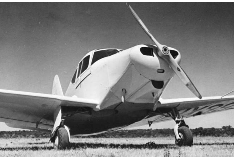
Aeronca Arrow prototype, NX39581, was powered by a 90-hp Franklin 4-AC-199-3. This aircraft, constructed of thin plywood, was lost in a crash after a propeller failure during a demonstration flight. (Photos from Aeronca: A Photo History , by Hollenbaugh & Houser)
