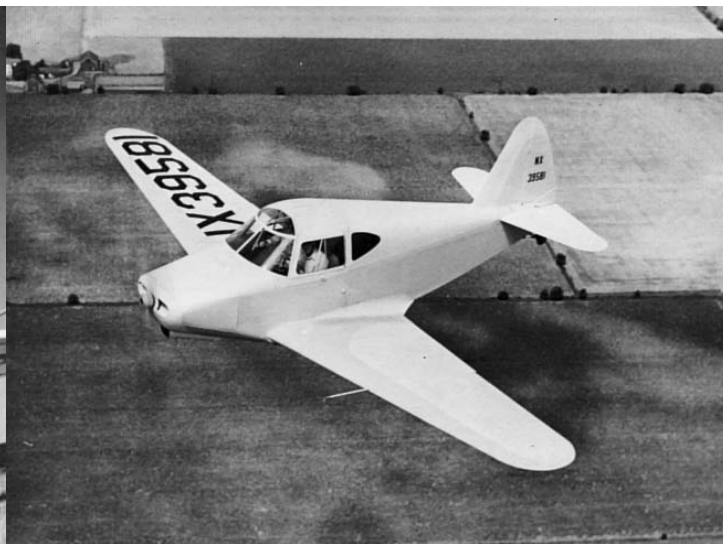
Aeronca Arrow prototype, NX39581, was powered by a 90-hp Franklin 4-AC-199-3. This aircraft, constructed of thin plywood, was lost in a crash after a propeller failure during a demonstration flight. (Photos from Aeronca: A Photo History , by Hollenbaugh & Houser)
