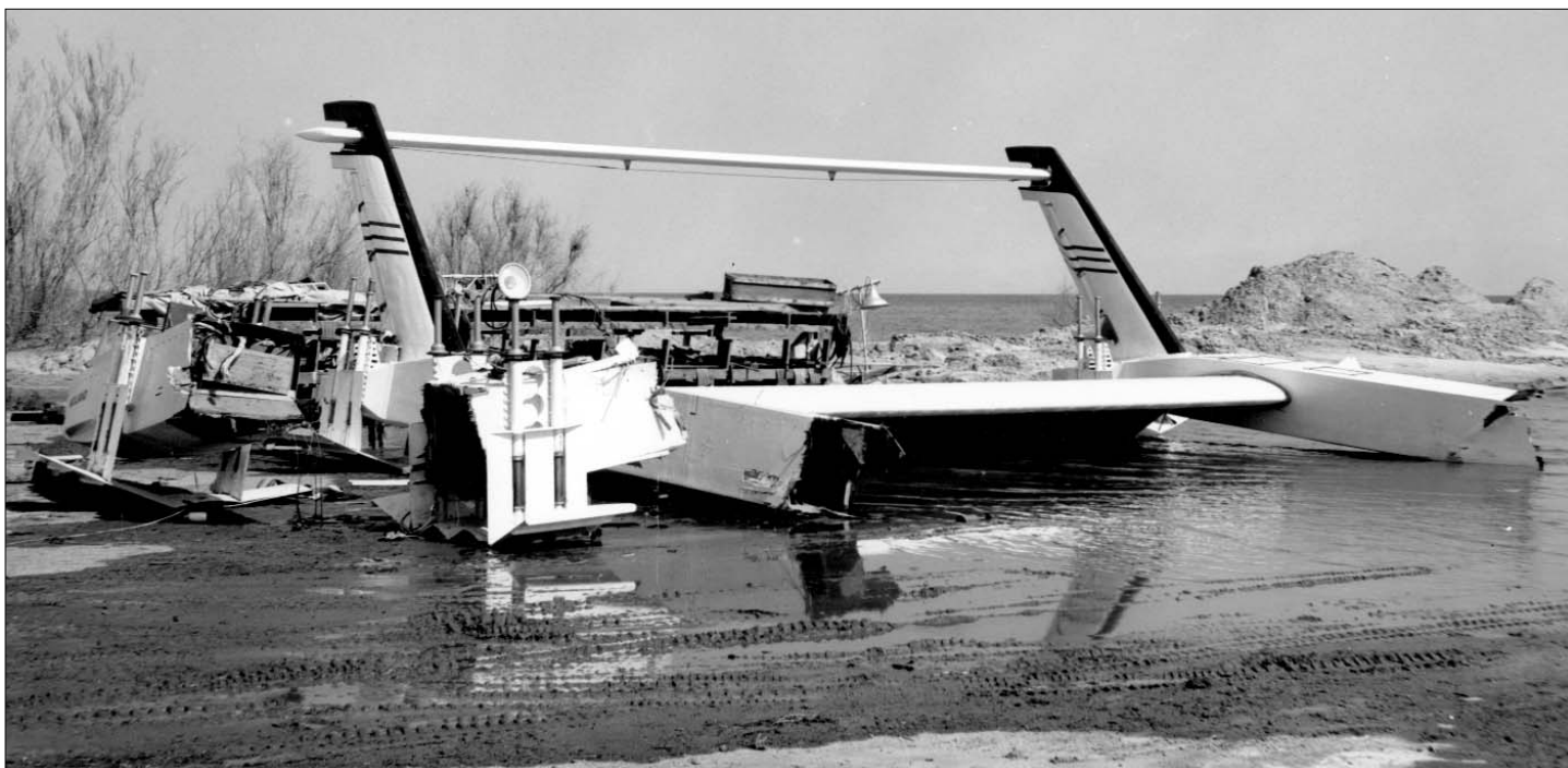
Remains of the Weilandcraft after departing stable conditions during flight testing. (Douglas photo from the author's collection)
