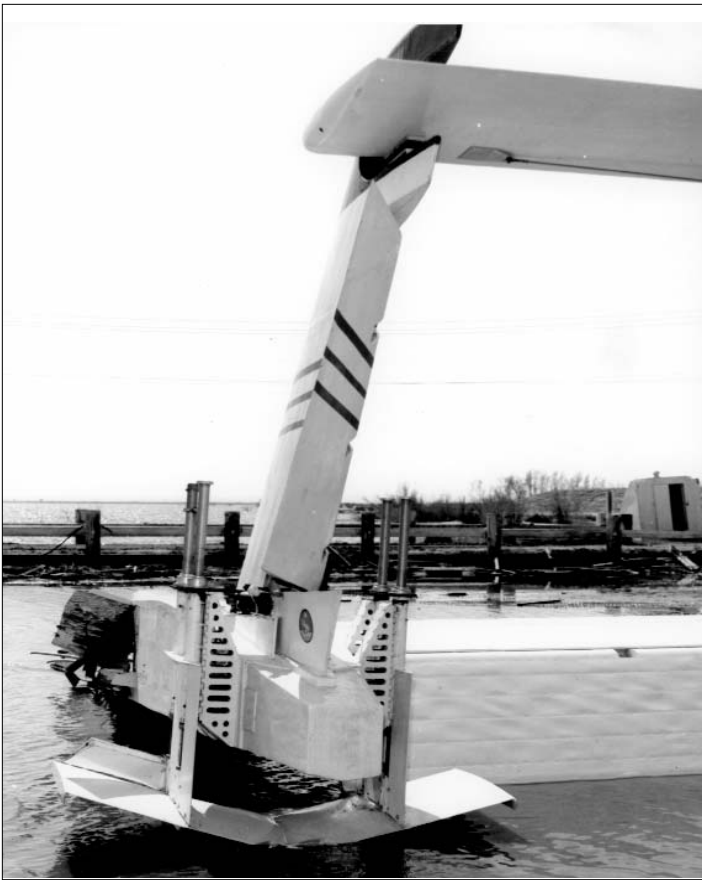
View showing the details of the aft hydrofoil skis on the destroyed craft. (Douglas photo from the author's collection)
