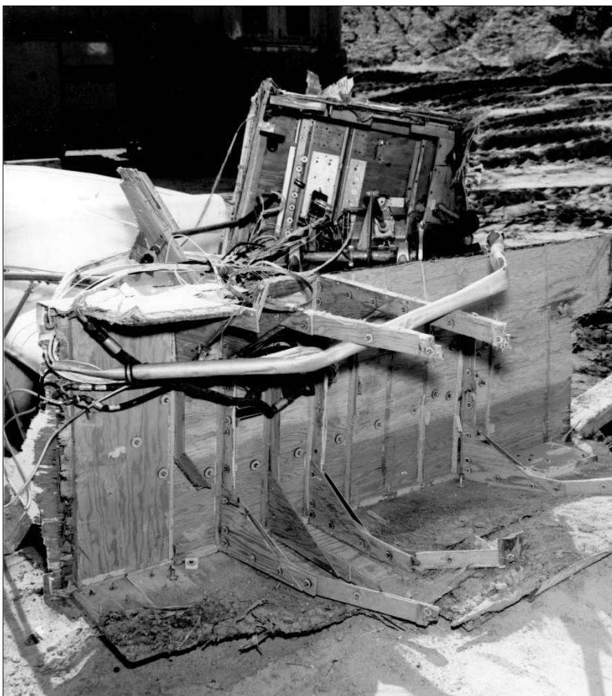
Another view of the engine pylon showing details of structural failure resulting from the crash. (Douglas photo from the author's collection)
