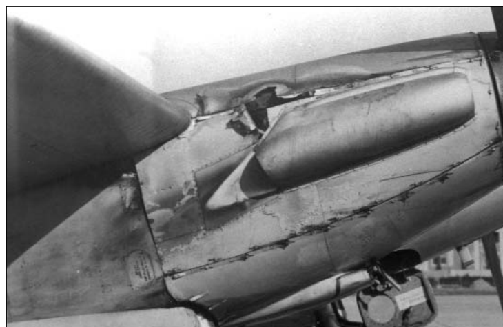
Damaged cowling and exhaust shroud of KB300 after overheating during March 31, 1943, flight test. (Photo from the NARA collection)
