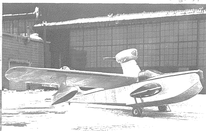
GA-1 Modified, with 125 H.P. engine and cantilever pylon.
