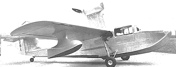
GA-2 Original GA-2 prototype with downward exhaust stacks and non-faired landing gear.
