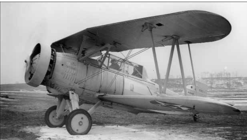
Curtiss O2C-1 Helldiver, Bu No. A8945, U.S. Navy. The enclosed cockpit was rare. The plane was powered by a Pratt & Whitney R-1340-4 rated at 450 hp. The date of the photo is March 20, 1932, the location is the Municipal Airport at Akron, Ohio.
