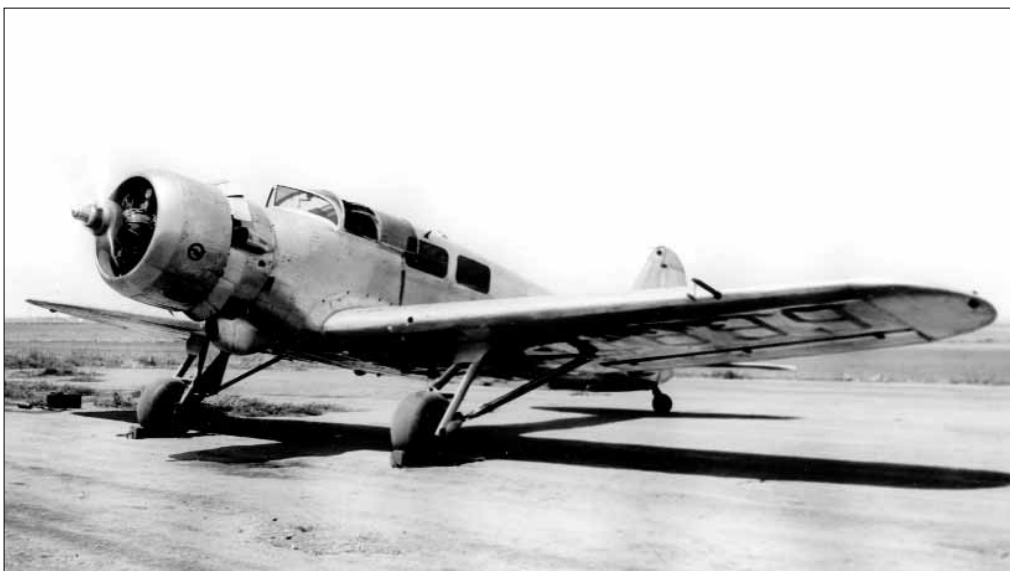
Left: The Vance-Dallas Model 1, NR12899, c/n 1, powered by a Pratt & Whitney Twin Wasp R-1830. Emil made this photo at Van Nuys Airport, Calif., on August 23, 1936.
