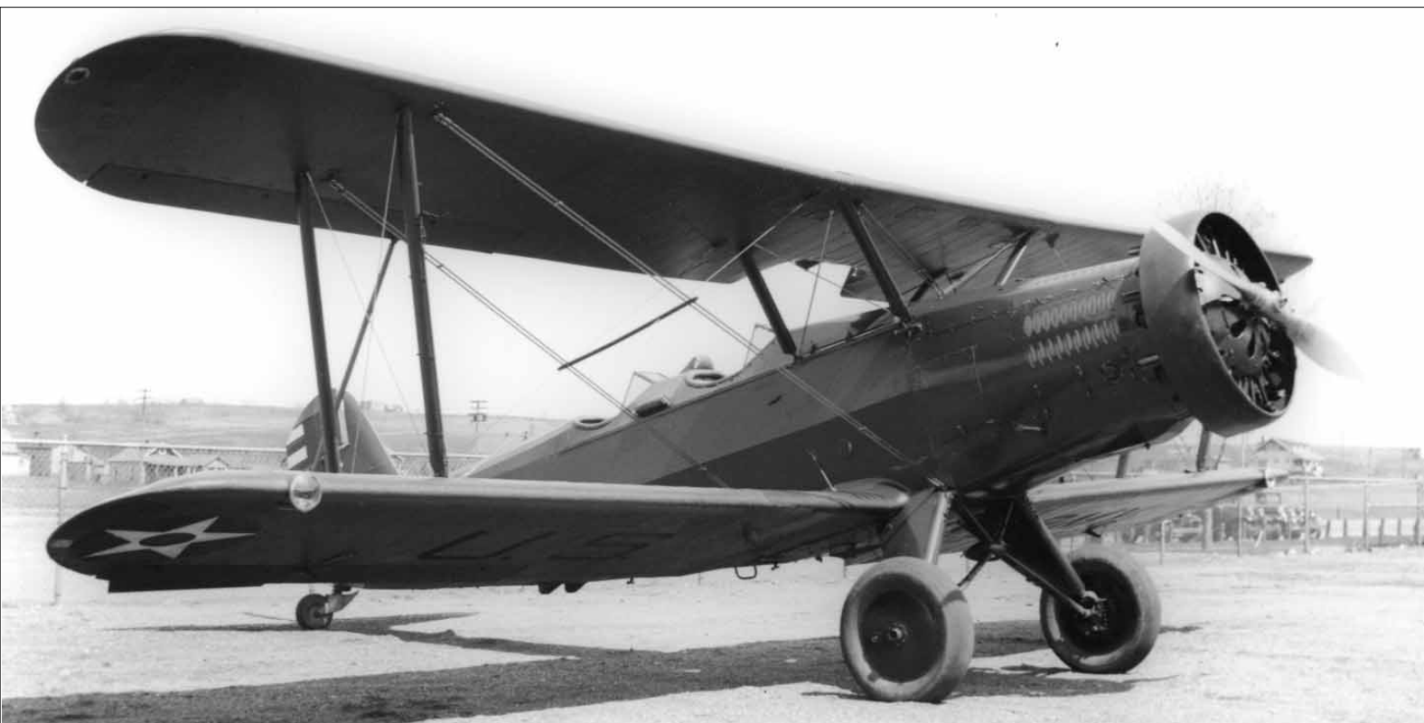
Above: Douglas BT-2A basic trainer of the U.S. Army Air Corps. During 1930, 30 Douglas O-32A Observation aircraft were converted to BT-2A Basic Trainers. A Pratt & Whitney R-1340-11 rated at 450 hp powered the BT-2A.
