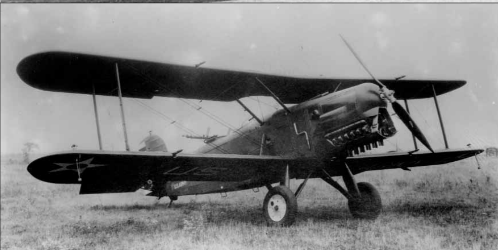
Above: Douglas BT-2A basic trainer of the U.S. Army Air Corps. During 1930, 30 Douglas O-32A Observation aircraft were converted to BT-2A Basic Trainers. A Pratt & Whitney R-1340-11 rated at 450 hp powered the BT-2A.
