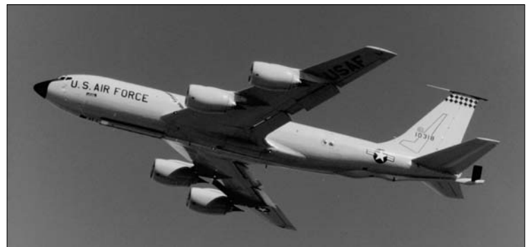
KC-135R, 61-0318, just after gear retraction. The huge CFM56 engines help quickly identify this model Stratotanker. (USAF photo from the author's collection)
