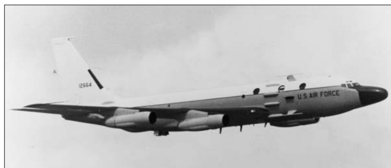
RC-135S, 61-2664, assigned to the 6th SRW at Eielson AFB, Alaska. This early version had three large portholes, towel rack antennas on pylons and four sensor fairings forward of the wing. (E-Systems P-118790-3 from the author's collection)
