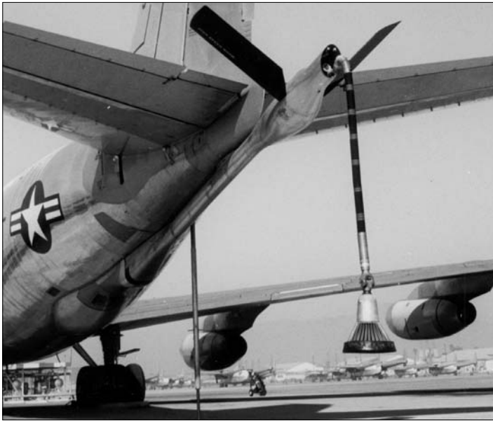
To permit refueling of early TAC fighters and USN/USMC tactical airplanes, Boeing developed the drogue adapter that could be attached to the boom nozzle. This system is also used to refuel airplanes from Allied air forces. (USAF photo from the author's collection)
