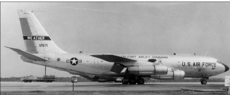
Ex-MATS C-135Bs were modified into WC-135Bs for use by the Air Weather Service. This May 25, 1972, photo shows the aircraft while still in its natural metal finish. (USAF photo from author's collection)
