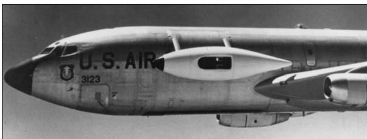
EC-135N, 55-3123, with ALOTS pod suspended from the main cargo door, housing a telescope that was used with the C-135B TIRA. (Boeing P40912)
