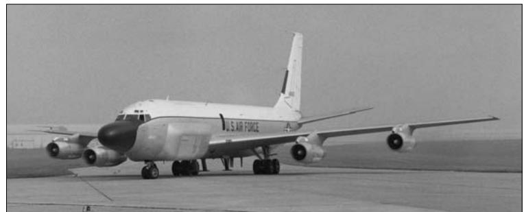
This hog-nosed RC-135M, 61-4843, of the 55th SRW reveals its Martin Aircraft sensor cheeks along with a plethora of other antennas. (via SAC Combat Crew Magazine from the author's collection)
