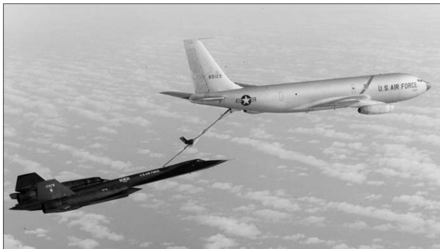
A 456th BW, KC-135Q refuels a Lockheed SR-71A, 64-17978, named "Rapid Rabbit" on a mission in Southeast Asia during the Vietnam conflict. The SR-71 was severely damaged in a landing accident July 20, 1972, and scrapped. (From SAC Combat Crew Magazine from the author's collection)
