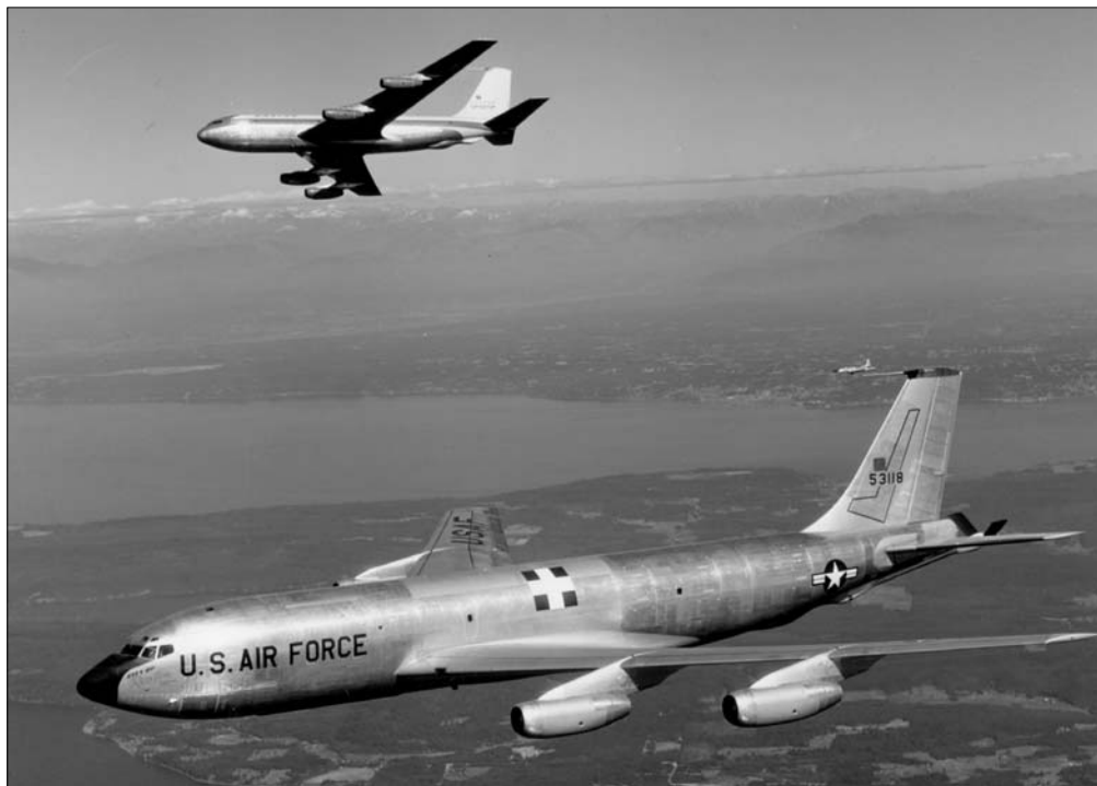
Here, the Model 367-80, fitted with the refueling pod, peels away from first KC-135A, 55-3118. The latter was named "City of Renton" and served in the test fleet until being converted into an EC-135K and transferred to TAC where she served as a command and control airplane. (Boeing)
