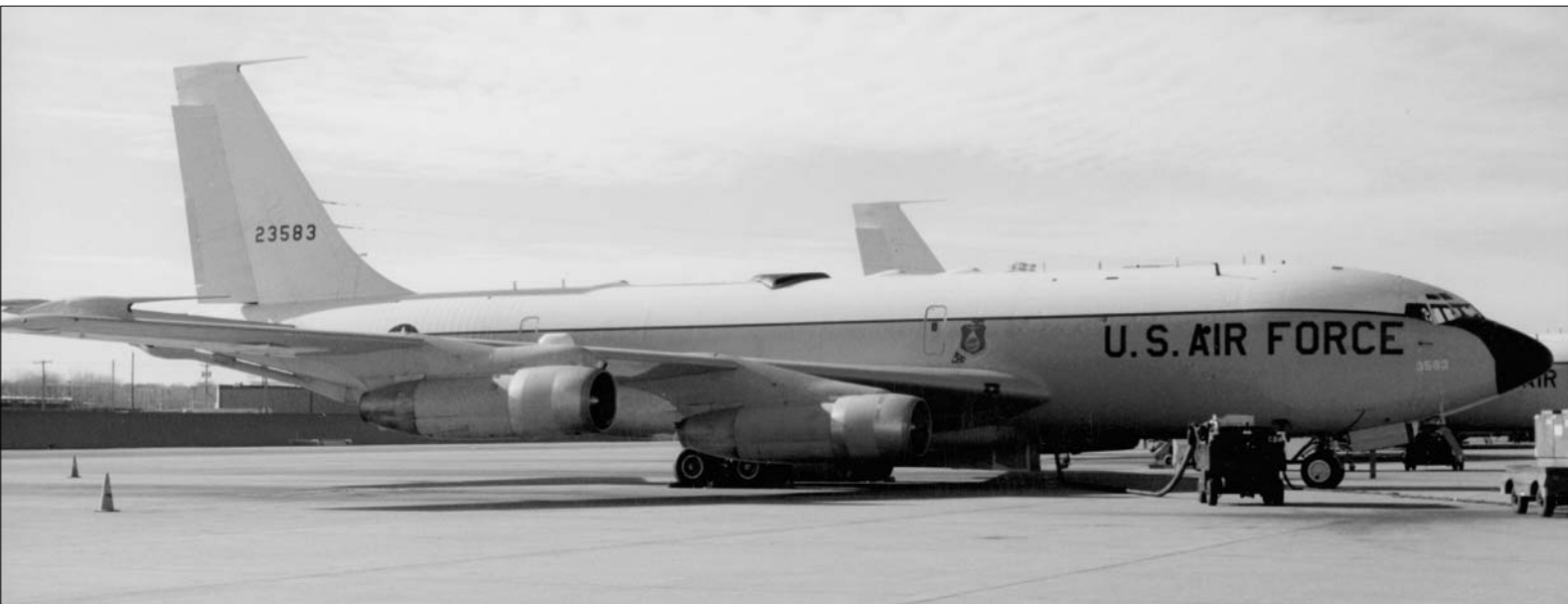
EC-135C, 62-2583, was assigned to the LOOKING GLASS mission with the 2nd ACCS, 55th SRW, Offutt AFB, Neb. Note the HF probe antennas on the vertical fin and on top of the wing tip. A saddle-shaped SATCOM antenna is mounted over the mid-fuselage. A pair of low-frequency long-wire antennas extend between the fin leading edge and short masts aft of the cockpit. (Photo by the author)
