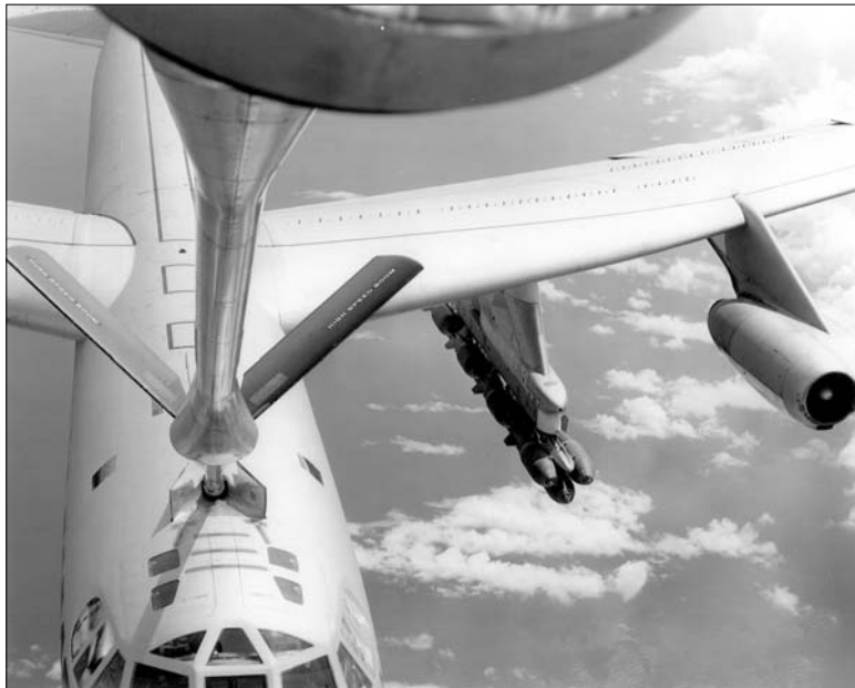
A Boeing B-52 taking on fuel while outbound on an ARC LIGHT mission over Southeast Asia. Up to 12 750-lb. bombs were carried on each external pylon, while another 27 bombs were carried internally. (USAF photo from the author's collection)
