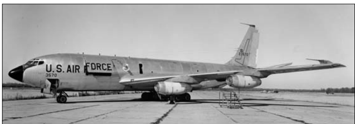
EC-135G, 62-3570, reveals its overwing HF probe antenna and the four additional blade antennas on top of the fuselage. (E-Systems P-4819-1)
