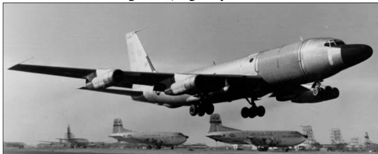
The sole RC-135E, assigned to the 6th SRW is distinguished by several features: thimble nose, fiberglass forward fuselage (right side only) and pods between the inboard engines and wing roots. (E-Systems photo from author's collection)
