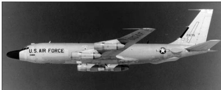
RC-135M, 62-4125, showing the static boom probe on the left wing tip, faired over boom position, additional blade antennas beneath the wing center section and thimble nose among characteristics of this model. (Kirby Kasen from the author's collection)
