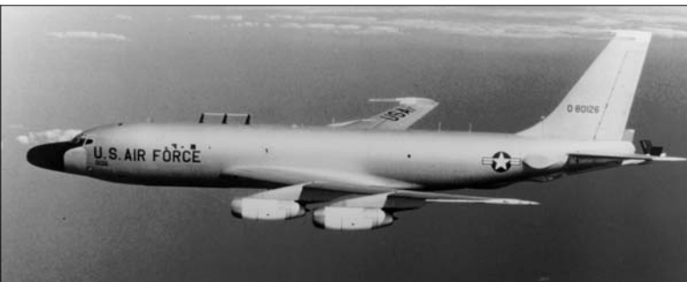
"Cobra Jaws" was RC-135T, 58-0126, equipped with a 2 segment LORAN antenna mounted on top of its fuselage, a hog nose, over-wing HF antenna on right wing and static probes on the wing tips along with other modifications. (SAC Historian from the author's collection)
