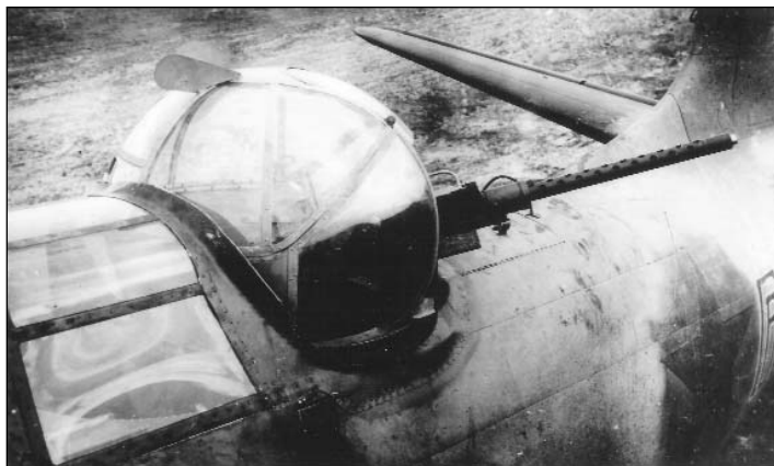
Close up of MV-3 turret on A-20B. This installation, in lieu of single flexible .50 caliber machine gun, was used operationally on many A-20Bs and early (pre-20) G models.
