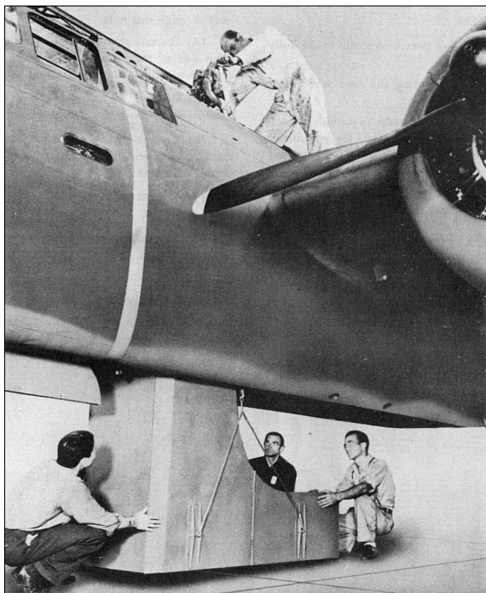
Removing 260-gallon forward bomb bay fuel tank. (From Douglas A-20B Maintenance Manual)
