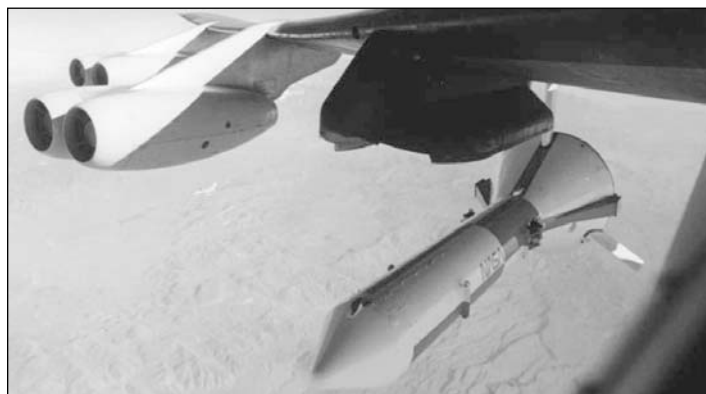
The SRB/DTV falls away from the NB-52B on July 19, 1984. (NASA photo EC90-0111-2)
