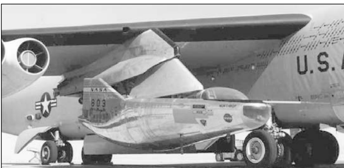
Northrop M2-F2 hangs from the Northrop Norair adapter on the pylon of the NB-52B. (NASA photo E13868)
