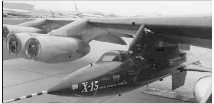
X-15-1 on the pylon of the NB-52B in late 1959. (NASA photo E5087)
