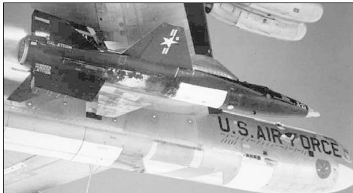
NB-52B carries Major Robert White in the X-15-2 equipped with the XLR-99 engine on an aborted attempt to launch the first flight with the "hot nose" on February 21, 1961. Nose art depicts an Eagle dropping an X-15 and the name "Challenger." (NASA photo E8698)
