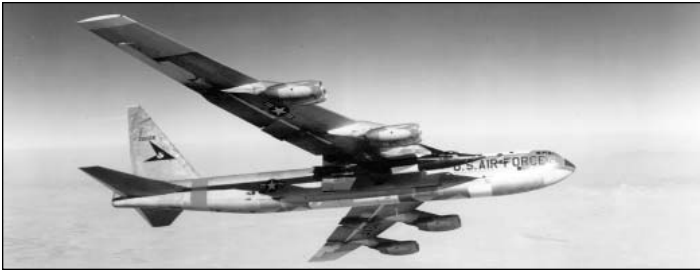
The NB-52B carries the X-15-1 in September 1960. The Day-Glo orange has been stripped from the vertical stabilizer. (Photo by Tony Panopolis)
