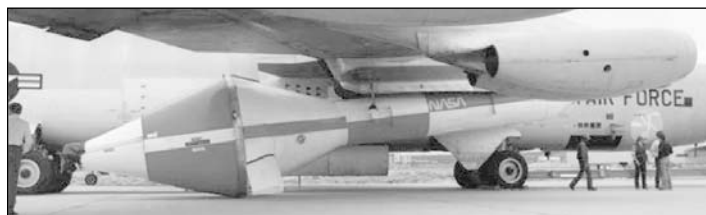
The SRB/DTV rest on the ground after the failure of the NB-52B pylon hooks on February 23, 1983. (NASA photo EC22788)
