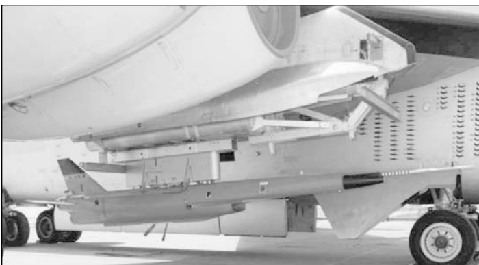
Firebee II drone hangs from the NB-52B pylon in 1977. (NASA photo EC7401)
