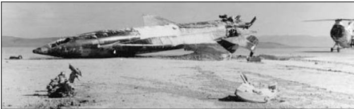
The X-15-2 lies on its back on Mud Dry Lake following Jack McKay's landing accident on November 9, 1962. (Photo from AAFTC/HO)
