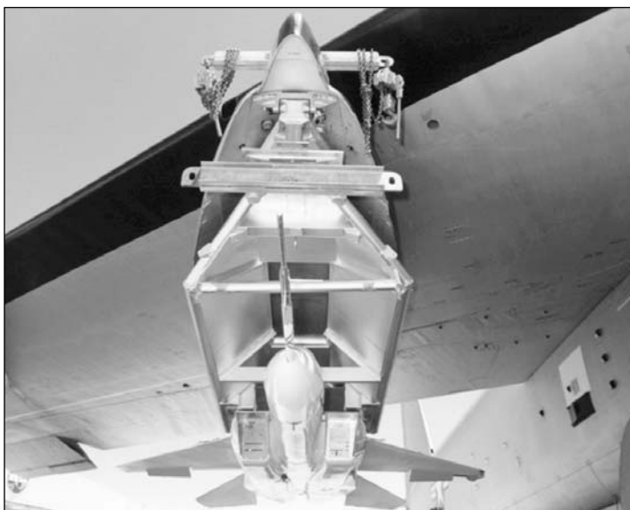
The 3/8-scale F-15 RPRV hangs from its adapter on the NB-52B pylon in April 1973. (NASA photo EC3644)
