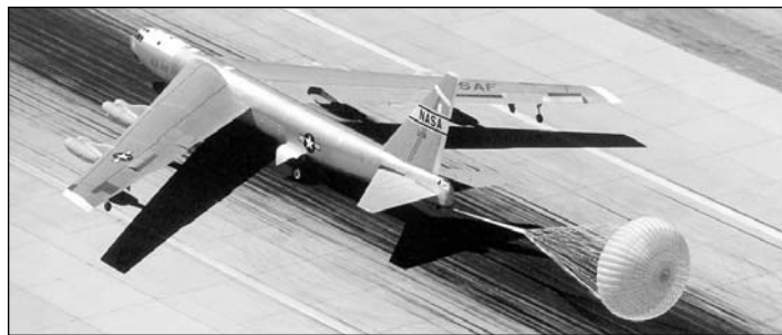
NB-52B tests the Space Shuttle drag chute on the concrete runway on September 27, 1990. (NASA photo EC90-262-27)
