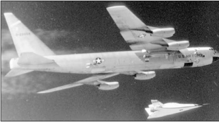
The X-24B falls away from the NB52B in 1975. (Photo by Bob Dorr via Greg Spahr)
