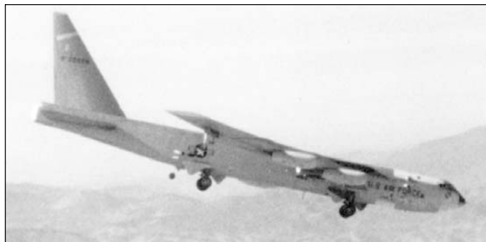
The NB-52B simulates the diving approach of the Space Shuttle in early 1970. (NASA photo E21203)
