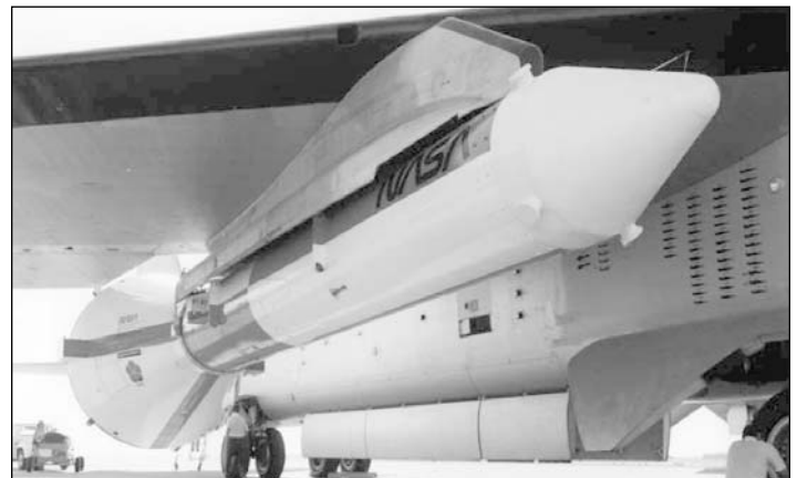
The Shuttle Reusable Booster Drop Test Vehicle hangs from the pylon of the NB-52B on June 17, 1977. (NASA photo EC7515)
