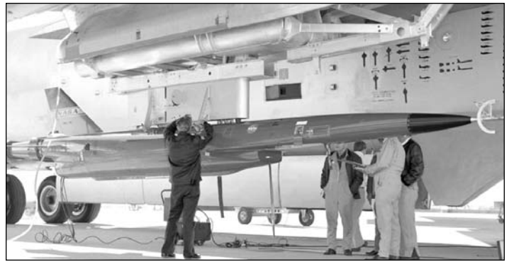
Blue Streak drone equipped with white Instrumented Standard Wing hangs from the NB-52B pylon in March 1979. (NASA photo ECN-10247)
