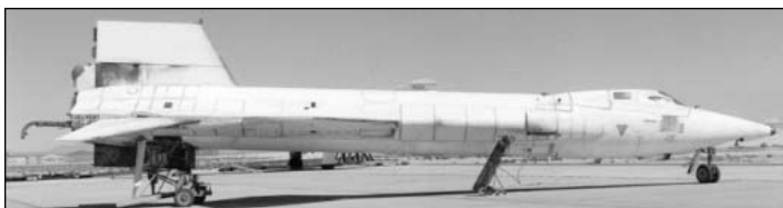
The scorched X-15A-2 following the all-up flight in October 1967. (NASA photo EC1834)
