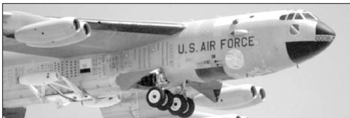
The NB-52B tests fuel additives with a pair of J85 jet engines mounted on a pallet in its bomb bay on June 30, 1995. (Author's photo)
