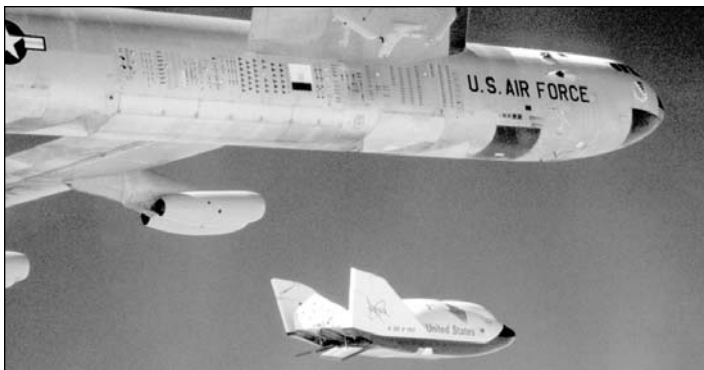
The X-38 V-132 falls away from the NB-52B on July 9, 1999. (NASA photo EC99-45080-25)
