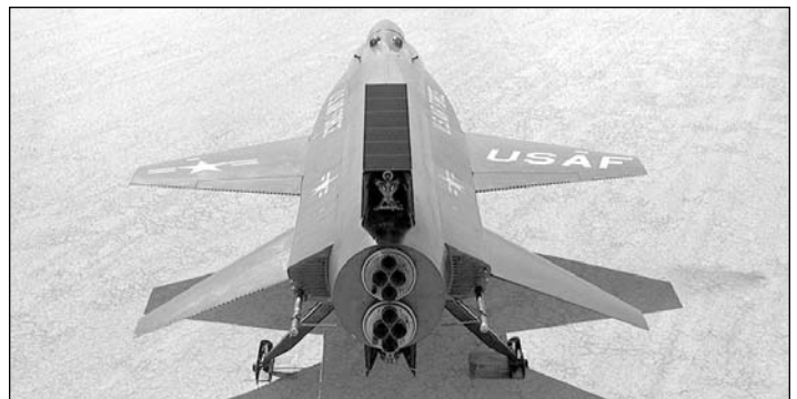
X-15-1 equipped with a pair of Reaction Motors XLR-11 engines sits on Rogers Dry Lake in 1960. (NASA photo E-5256)
