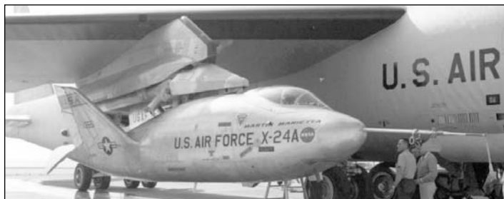
The X-24A hangs from its adapter on the pylon of the NB-52B on May 8, 1969. (NASA photo EC69-2196)
