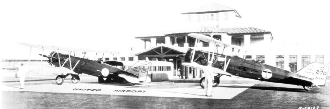
Above: At United Airport Burbank, California, are two Boeing 40s. The left aircraft is C179E of Pacific Air Transport named 'Baker,' after Mt. Baker. It is a Boeing 40C that has four passenger seats and flown on Air Mail Route 8 (CAM 8). The right aircraft is C270 a 40A converted to a two cockpit model, the aft mail pit is now a cockpit and the aircraft has only two passenger seats. This aircraft is used on Air Mail Route 18. (Photo from United Airlines Archives)
