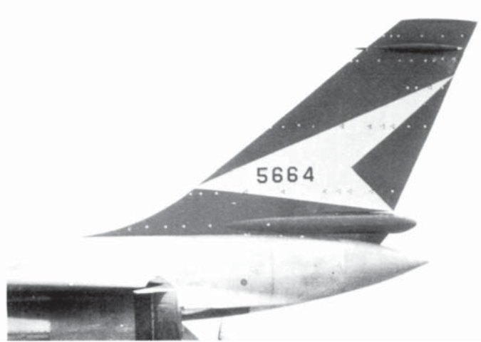
18/19: Two views of '5664's vertical tail. Strain gauge locations are readily discernible as each is marked with a colored triangle. Triangle pattern was mirrored on both sides of the fin and rudder.
