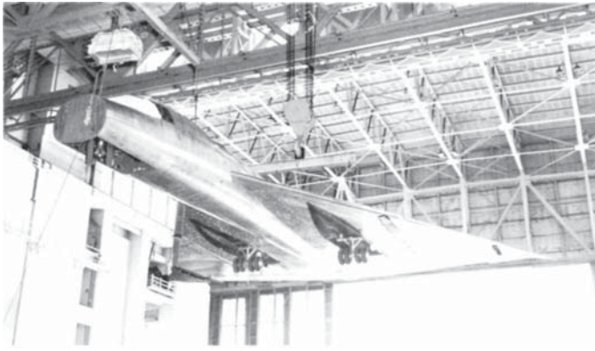
13: Moving B-58A airframe "number 4A" into the structural test facility on the Wright side of Wright-Patterson AFB, Ohio. Note the abbreviated landing gear for moving the aircraft on the ground. (Photo from Wright Air Development Center)
