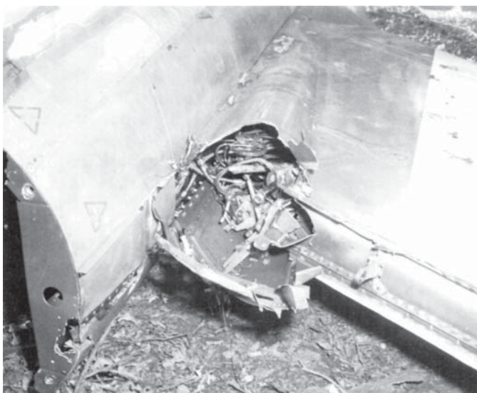
7: The hydraulic actuator assembly for the rudder was completely destroyed when the rudder separated from '5664's vertical fin at nearly twice the speed of sound. (Photo from General Dynamics)
