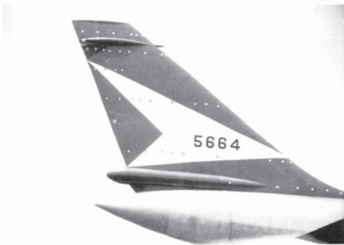
18/19: Two views of '5664's vertical tail. Strain gauge locations are readily discernible as each is marked with a colored triangle. Triangle pattern was mirrored on both sides of the fin and rudder.
