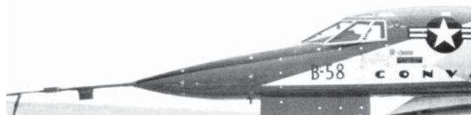
16: Nose of '5664 with strain gauge locations marked by triangles. Color scheme was primarily red and white.
