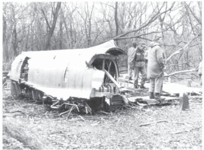
8: '5664's aft center fuselage section with right wing panel partially attached. Severity of damage underscored how completely the airplane was destroyed as a result of the enormous aerodynamic loads imposed at 2.0 Mach. (Photo from General Dynamics)
