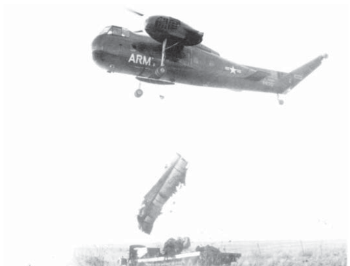
9: Workhorse of the parts location and retrieval team was a single Sikorsky H-37. Its heavy lift capabilities allowed it to haul the biggest chunks of 5664, such as this engine nacelle component (note engine already on flatbed), to the truck and trailer units tasked with transporting everything back to Ft. Worth. (Photo from General Dynamics)
