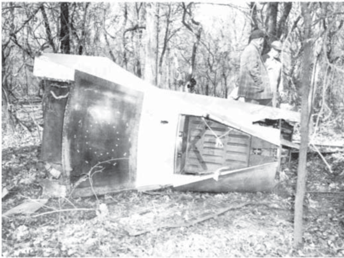
6: Empennage and vertical tail of '5664 as it was found in a field outside Duncan, Oklahoma. Telemetry antenna for the data relay system was located inside the area covered by the black dielectric panel with the circular pattern on it. Triangles mark points where strain gauges were located. (Photo from General Dynamics)
