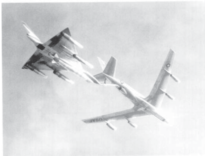
2: At one point in its flight test career, '5664 was utilized to clear the B-58's inflight refueling envelope. It is seen taking on fuel from an early, short-tail KC-135A. (Photo from General Dynamics)
