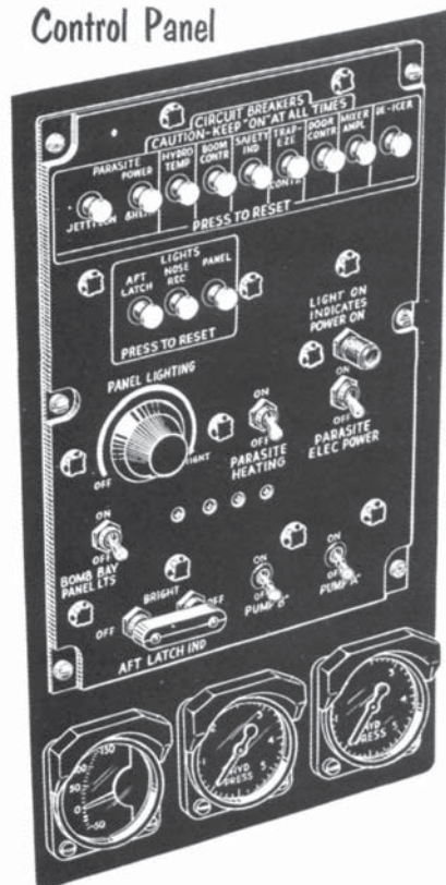
Trapeze Operator's Auxiliary Control Panel Diagram from the Utility Flight Handbook for the GRB-36DIII Featherweight Configuration III/RF-84F Composite Aircraft. (Roger Crippliver)
