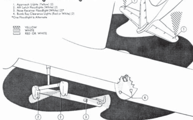
Exterior Lights Arrangement Diagram from the Utility Flight Handbook for the GRB-38D-III Featherweight Configuration III/RF-84F Composite Aircraft. (Roger Cripliver)
