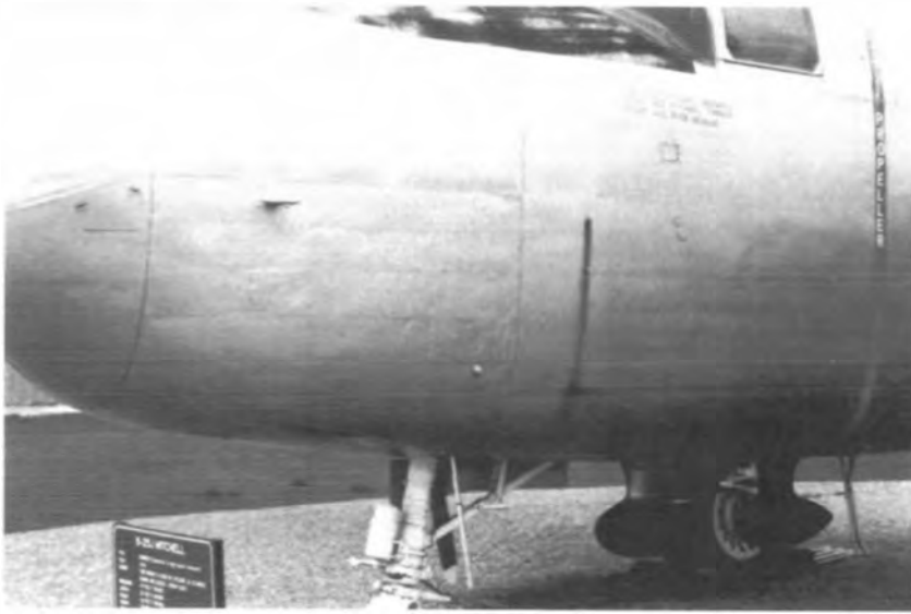
Left: The nose of the B-25J was flared over.
