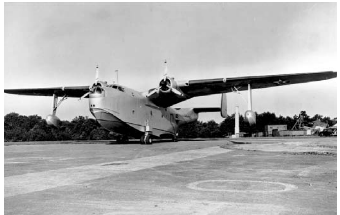
Martin XPBM-1 prototype note the horizontal tail with no dihedral. This was the only Mariner with this feature. (Photo USN/Martin via Bruce Barth)
