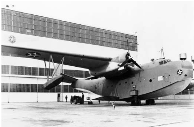
Martin PBM-3 at the Martin plant in early WWII. The big flying boat was powered by Wright R-2600- 12, 14 cylinder engines of 1700 hp. (Martin photo from the A. Hansen collection)
