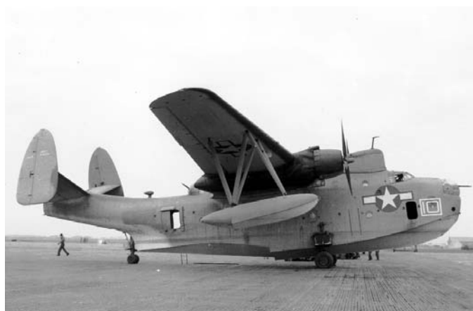
Martin PBM-5, Bu59295 was equipped with the Pratt and Whitney R-2800-22 18 cylinder engines of 2100 hp. The PBM-5s superior speed, range and payload made them a more effective patrol aircraft especially in the Pacific War. (Peter M. Bowers collection from A. Hansen)
