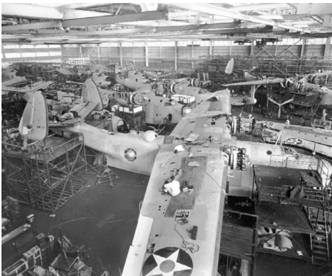
Martin PBM-1 production line at the Glenn L. Martin plant near Baltimore, Maryland in 1940. Deliveries of the first 21 production PBM-1s started in September, 1940. (Martin photo 20481 from the R.D. Neal)
