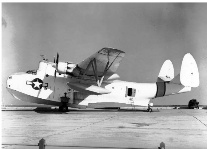
This Martin PBM-3S incorporated British anti-submarine color scheme, white with gull gray top surfaces. The -3S omitted armor and power turrets for longer combat range. (Peter M. Bowers collection via A. Hansen)
