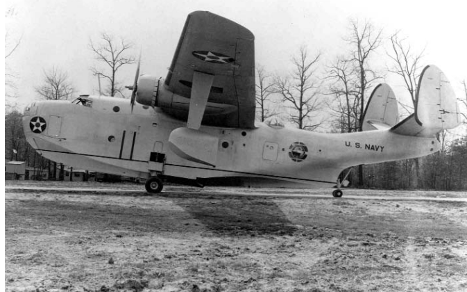
Martin XPBM-2 (Bu.No. 1247) Shown at the factory April 15, 1941. Note dihedral of the horizontal stabilizer with verticals normal to the horizontal stabilizer. This was taken from the PBM-1 and converted to a Navy strategic bomber with increased bombloads and fuel. It was also designed to be catapulted from barge. (Photo USN/Martin via Bruce Barth)
