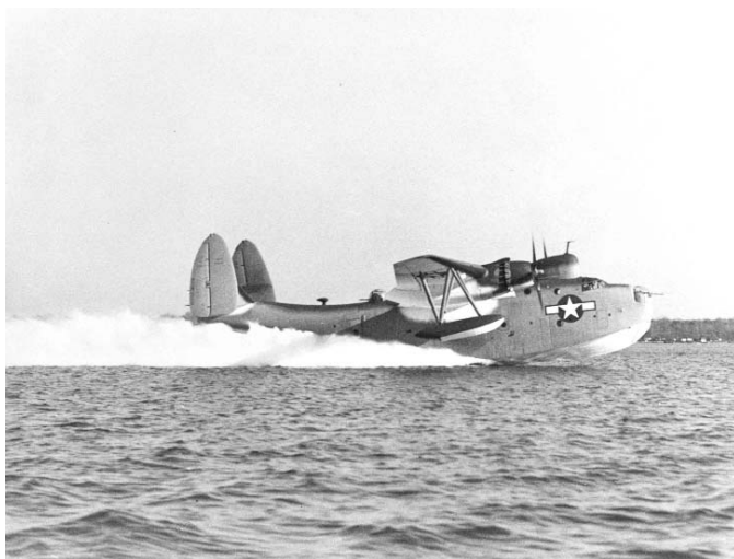
Martin PBM-5 Mariner taking off from smooth water. The large Structure just aft of the cockpit is the surface search radar. (Photo USN/Martin via Bruce Barth )
