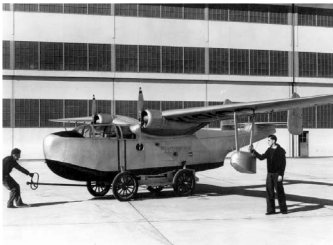
Martin Model 162A three-eighths scale flying model (N19168) "Tadpole Clipper" now in NASM Silver Hill facility. (Photo USN/Martin via Bruce Barth)
