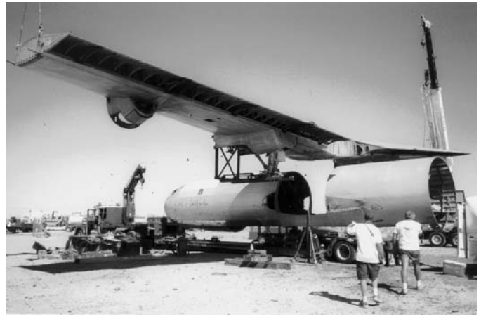
Above: After the Wing-center-cap was removed the wing assembly minus the engines, ailerons and flaps removed the wing can be lifted complete. Photo by, Wayne M. Gomes, Author, A.A.H.S. February 2000
