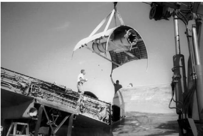
Above and below: The wing center cap is carefully lifted from the fuselage. This will allow the separation of the two forward sections and the center wing section. It took Worldwide Aircraft Recovery about 6 weeks to totally dismantle the B-29. It took 4 trucks and trailers three trips to deliver the aircraft to Wichita, and with out a scratch I might add. Photo by Cliff Gaston. U.S.A.M. March, 2000
