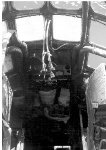
Above and right: The broken out and crazed glass over the pilot and copilots position gives testimony to the ravages of 43 three years of harsh desert dwelling that the aircraft was subjected to. It became a sanctuary for lizards, birds, and many other desert creatures. Photo by Wayne M. Gomes, Author. A.A.H.S. February 1998
