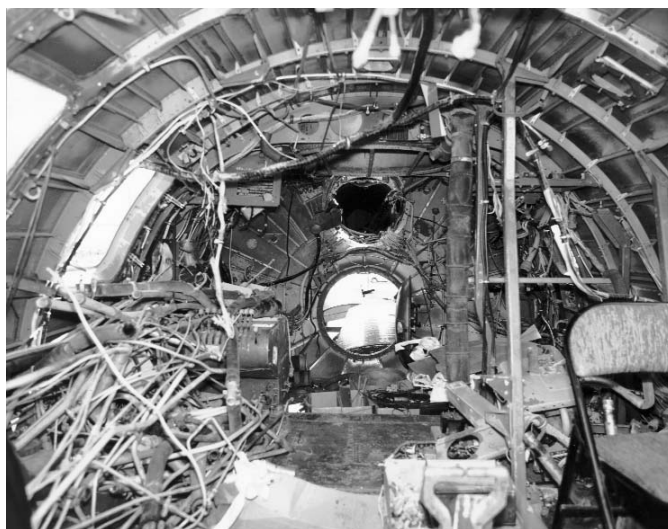
Above: A photo of the B-29 "Doc's" 41 section (nose section) as it looked after the 43 years old derelict sat on the Mojave Desert in California. (Note the Flight Engineer's station on the left). This photo was taken in May of 2000 when the B-29 first entered the Boeing Aircraft Company facility in
