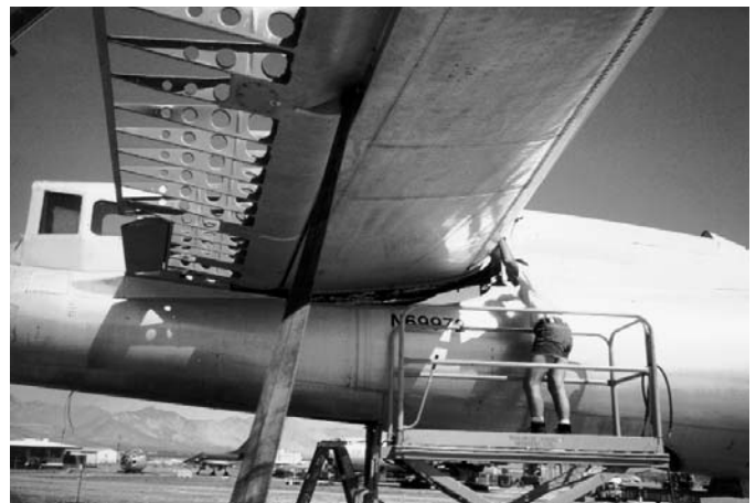
Below two photos: The Horizontal tail is removed from the aft section of "DOC" and put onto a support Cradle, that was designed to protect it in transit. The tail gunners compartment is in plain view. Note the fabric covering of the control surface has been rotted away. Photo by Cliff Gaston. U.S.A.M. March 2000
