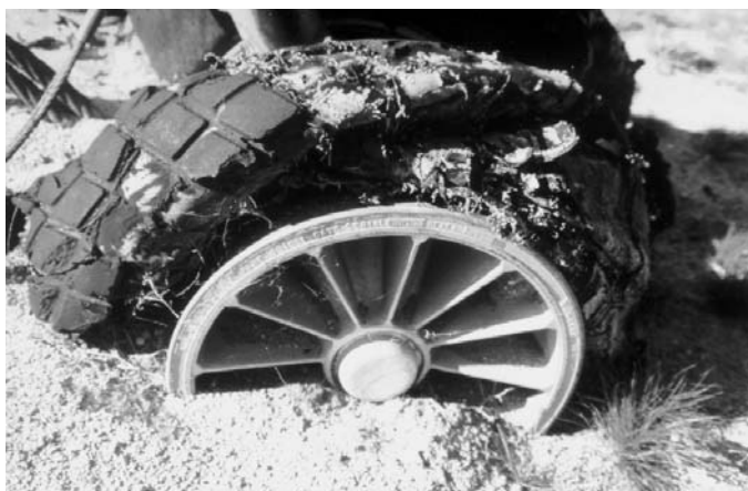
Above: The nose wheel is seen half submerged in the desert sand, where it had not moved for over 43 years. It took two tractor haulers and 9 shear pins, 4 days to pull the B-29 from its hole in the sand and tow it 38 miles to safety. Photo by, Wayne M. Gomes. Author. A.A.H.S. February 1998
