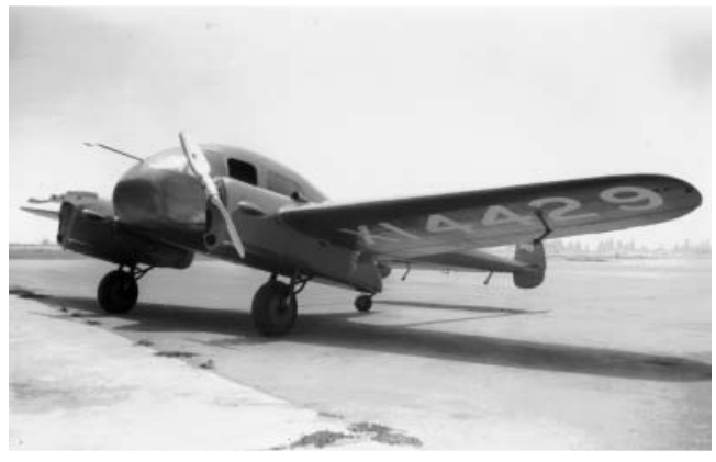
The American Gyro Crusader, AG-4, NX14429 with retractable landing gear. Emil took this photo at Grand Central Air Terminal, Glendale, on June 20, 1936. The Crusader had 2 Menasco C-4-S, 150 hp engines.
