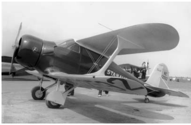
Beech B-17L, NC 12592, c/n 12 of Stanavo at the 1934 National Air Races at Cleveland on September 2, 1934. This Staggerwing had a Jacobs L-4, 225 hp engine.
