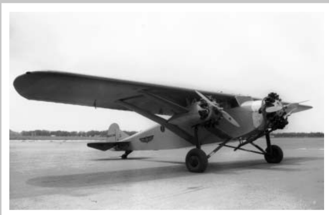
Bach 3-CT-9 trimotor , NC809M (19) of Union Air Lines, at Grand Central AirTerminal, Glendale, California, June 2, 1936. The nose engine is a Pratt & Whitney 450 hp and the 2 under-wing engines are Wright J-6 , R-760 , 225 hp engines.
