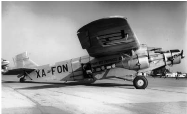
Ford 5-AT-D (103) of 1931, XA-FON, operated by Transportes Aereos de Jalisco and named Estrella Fugaz at Grand Central in 1948. The original engines were replaced with 3 Pratt & Whitney 985, 450 hp engines and cowlings from Vultee BT-13 trainers.
