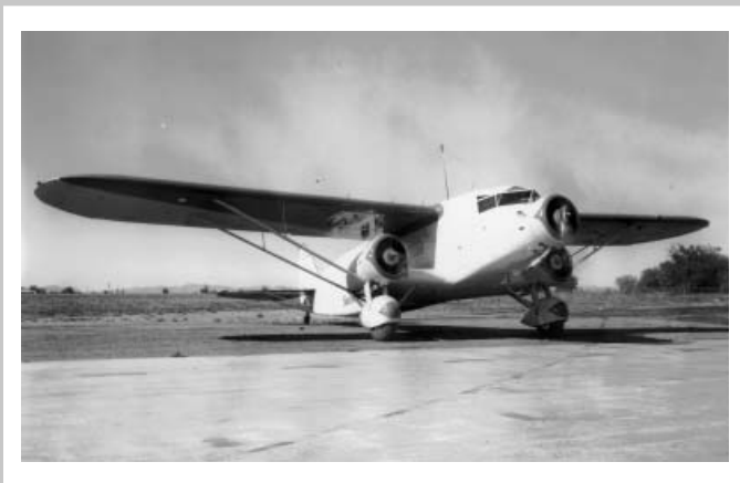
This Stinson U trimotor , NC 12196 ( s/n 9023) was operated by the San Francisco Examiner newspaper in the early 1930s. Three Lycoming R-680-BA, 240 hp engines powered the aircraft.
