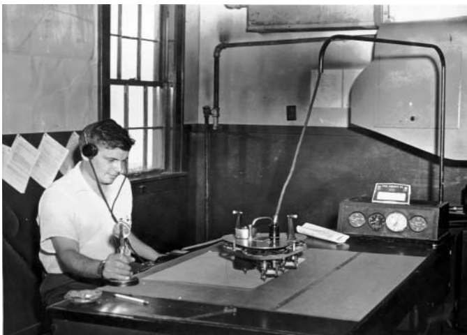
Above: Dick Hill at the Link Trainer desk during his years at Lewis College, Lockport, Illinois. One hand on the “mike” while watching the movement of the desk top “crab.” Note the nose of the extra trainer fuselage parked against the wall. (Photo from authors collec-
