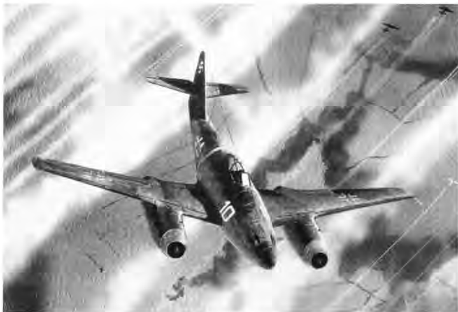
The revolutionary Messerschmitt Me. 262A-1a twin turbojet fighter with an operational airspeed of 540 mph (869 kph). Pictured here is "White 10" of III./EJG2 that was operational in early 1945. (Steve Ferguson, Messerschmitt Me. 262)
