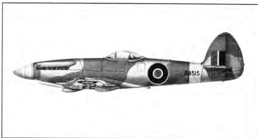
The successor to the famous Spitfire , the Spitfire , first production model RB515, similar to the fastest WWII piston-engine fighter, RB518, at 494 mph (795 kph) in level flight. This was the last piston-engined fighter produced by Supermarine and was too late to see action in WWII. (Bruce Robertson, Spitfire — The Story of a Famous Fighter )
