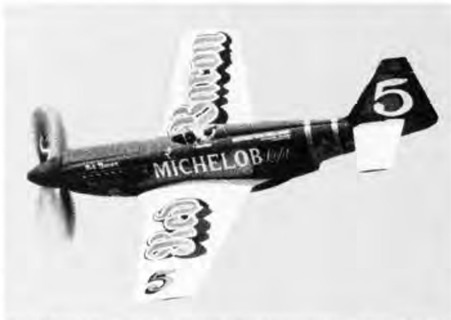
The Red Baron in-flight showing the enlarged vertical stabilizer and modified canopy. Note: The high pitch angle of the contra-rotating propellers. (Bruce Treadway, Air Classics)
