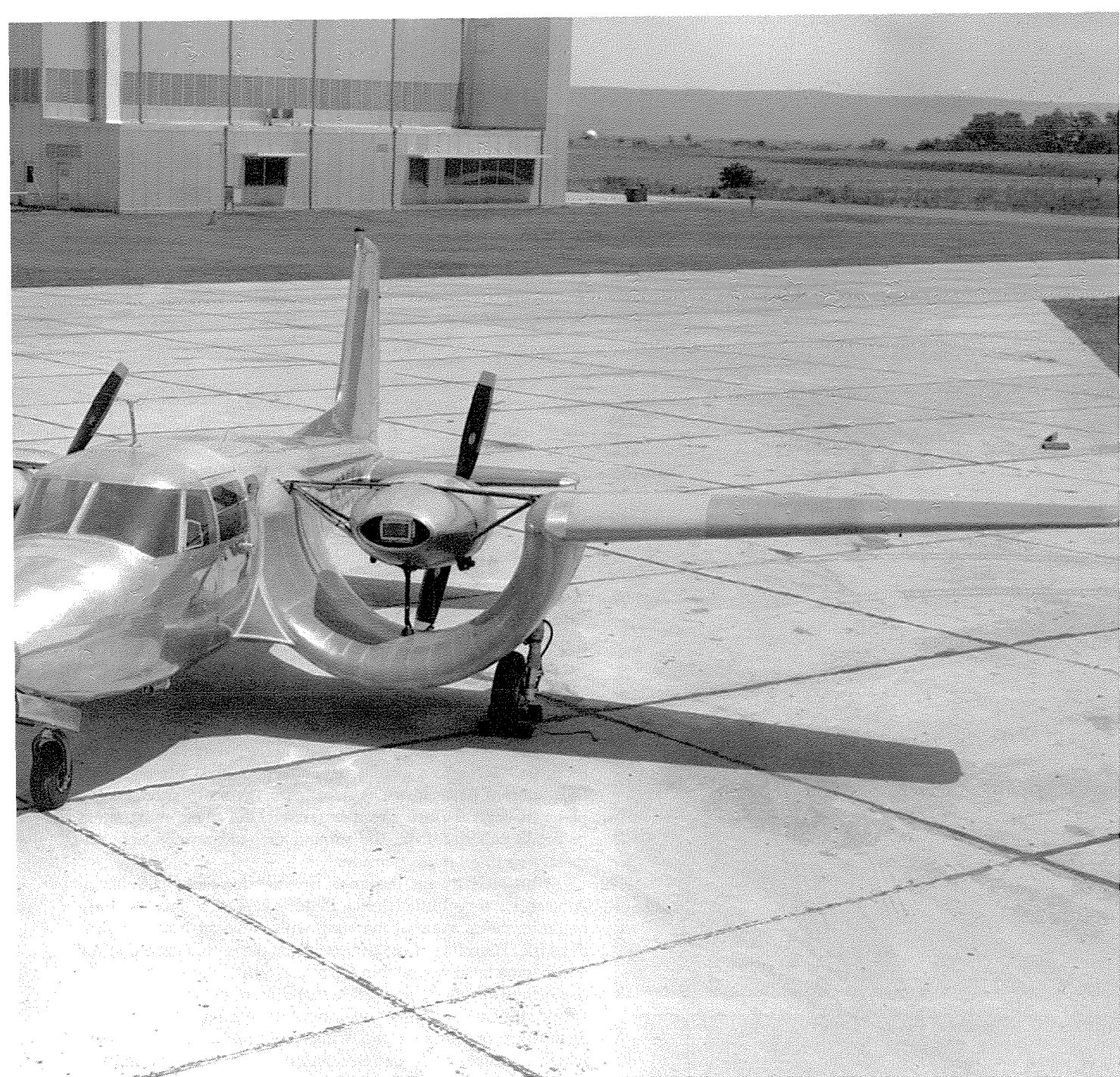
Above: The unpainted CCW-5 sits on the ramp at the Hagerstown, Maryland airport. Evident are the semi-transparent fiberglass inner channel skins. (Raup Photographic Studios, Author's Collection) Left: The second CCW-5 at Oxnard, CA 19 June 1953. Mr. Custer at right. (Photo by Harry Gann)
