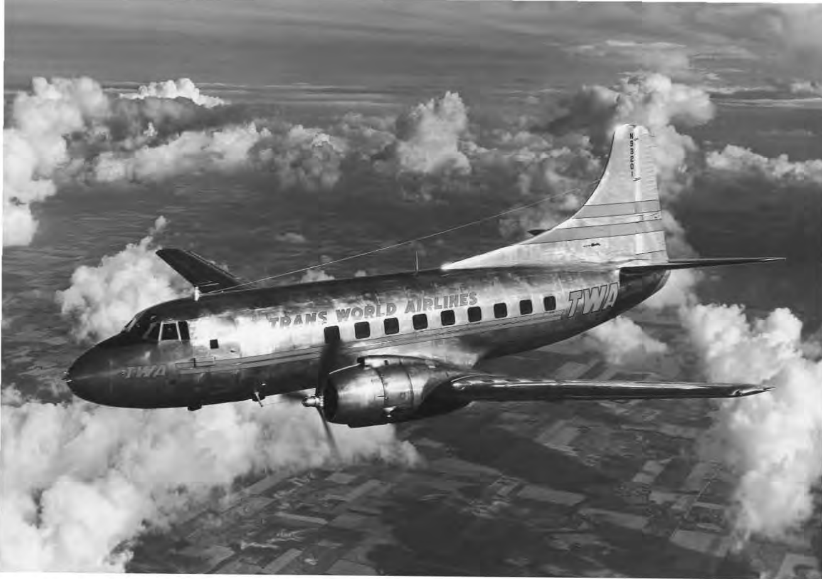
The Martin 202A, 404, Martinliners, used R2800-CB engines, using water injection and autofeathering for takeoff. The 202 grossed at 43,000 pounds, the 404 at 44,900, lengths 71 feet 7 inches and 74 feet 7 inches, wingspans 93 feet, 3 inches. (TWA photo from the Edward G. Betts Collection)
