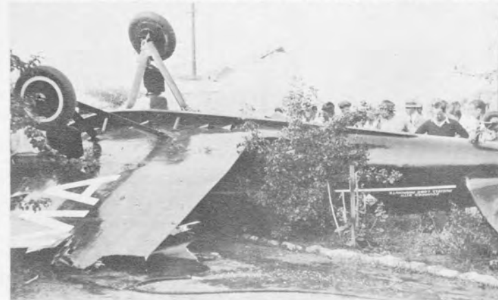
Herb Fahy crash after rudder failure -Moore
