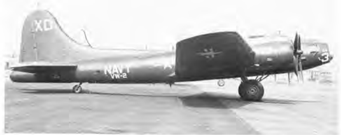
PB-1W BuNo 77236 with Navy Airborne Early Warning Squadron Two (VW-2) in 1954. The aircraft of VW-2 retained the markings of its predecessor squadron, VX-4. Note that the AN/APS-20 radar and bulbous radome were not installed in this PB-1W when this photo was taken.
