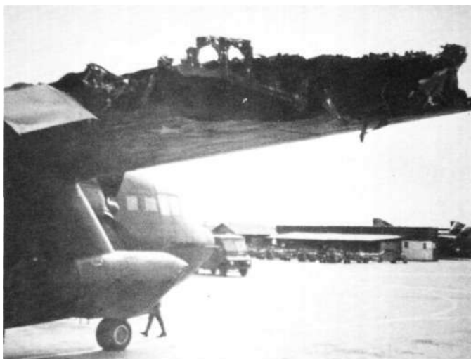
AC-119K 53-7883 lost half of the right wing to ground fire, but flew 180 miles for a safe landing. (U.S. Air Force Photo, Author's Collection)
